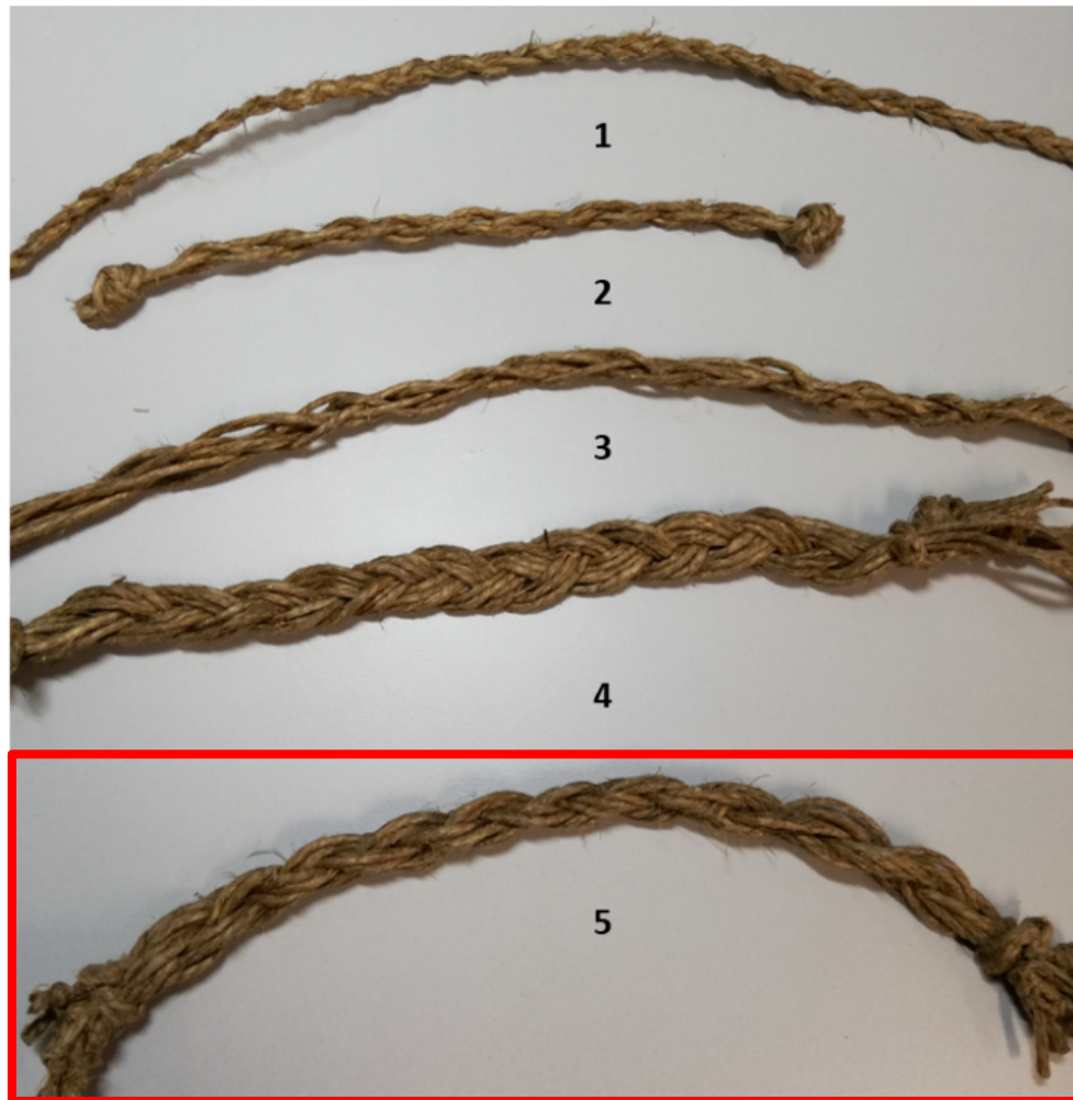
Prototype yarns created for better shape visualization. 1) 3x1, 2) 4x1, 3) 6x1, 4) 3x4 and 5) 4x3
