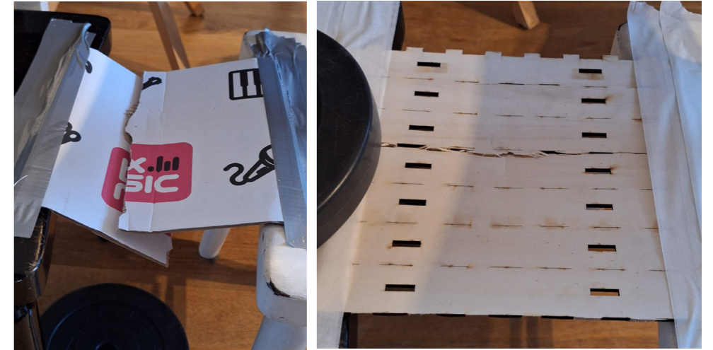
3.5kg of impact over 300mm Results: - Cardboard broken - Plywood broken
