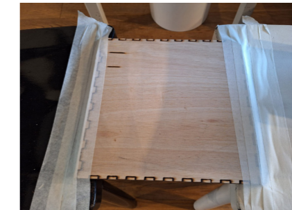
3.5kg of impact over 300mm for 9mm plywood Results: - Plywood intact
