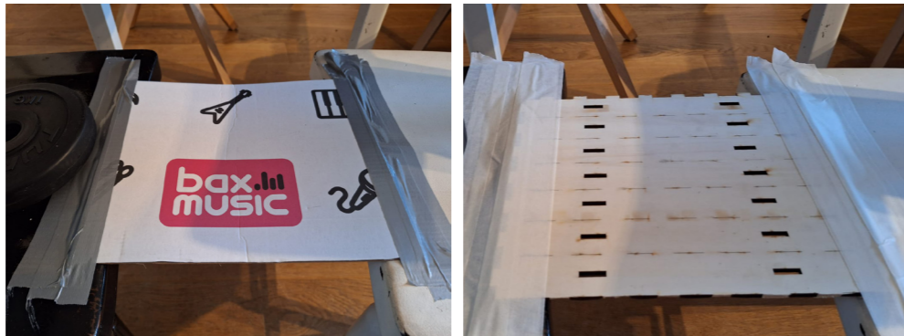
1kg of impact over 300mm Results: - Cardboard intact - Plywood intact
