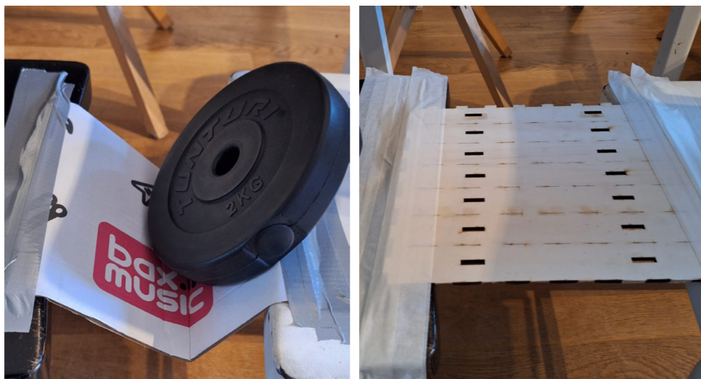
2kg of impact over 300mm Results: - Cardboard intact - Plywood intact
