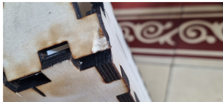
Figure 7.6.2: Transportation damage marks on packaging.
