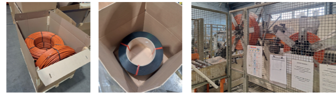
Figure 6.3.1.1: coiled PEX pipe in packaging, a roll of feuellard and the coiling machine used for PEX pipe packaging.
