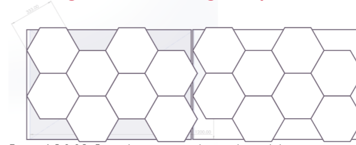
Figure 6.3.1.10: Protruding parts can be overlapped during transport to prevent trailer capacity loss.
