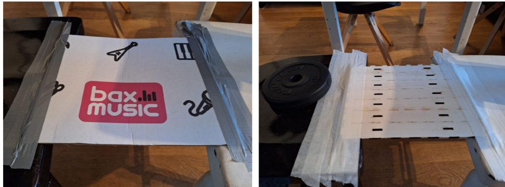
250g of impact over 300mm Results: - Cardboard intact - Plywood intact
