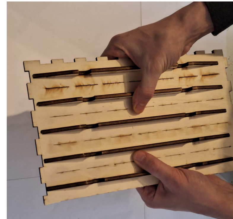
Figure 7.5.2.4: Breaking into rails element.
