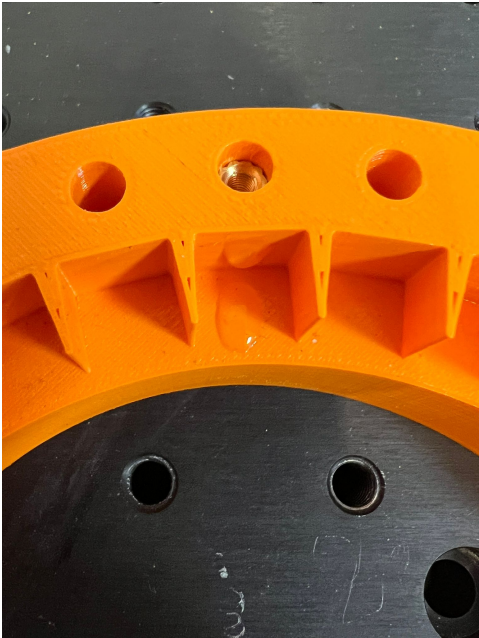
(a) Adhesive used in the assembly of individual magnets on the stator.
