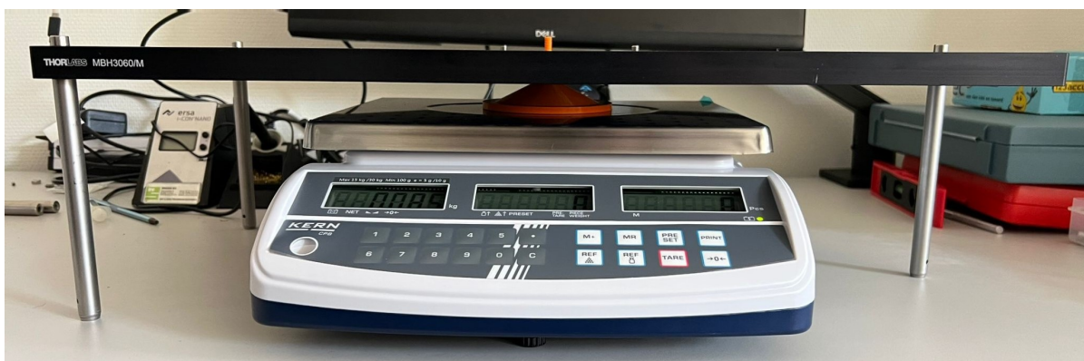
Figure 4.16: Raised base plate and scale mount - The scale mount allows for the Thrust Bearing Mount to be assembled onto its thread, thus bypassing the base plate and being entirely supported by the scale.
