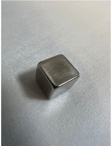
(c) Surface of the magnet after sanding and cleaning.
