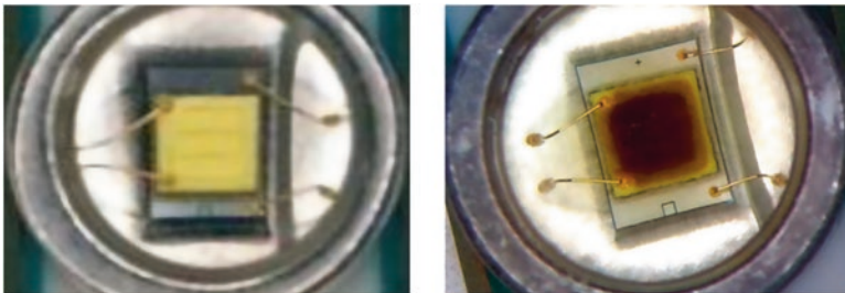
Fig. 8.3 Influence of thermal aging on the discoloration of LED optical package [47, Reproduced with permission from authors]
