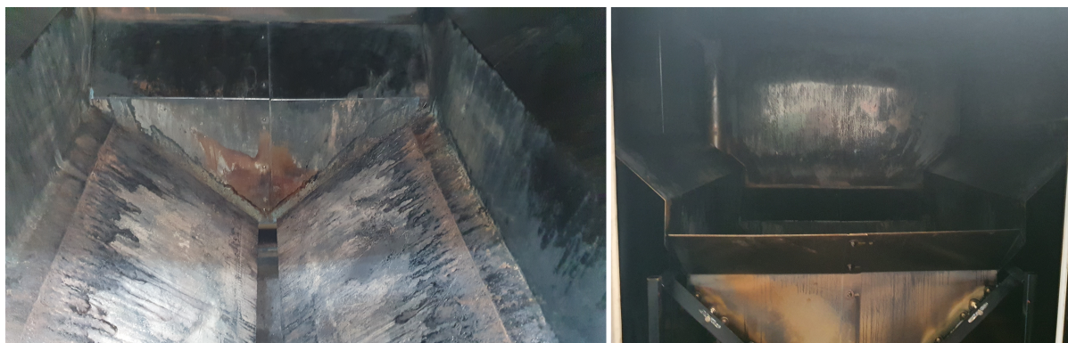
Figure 1.1: The Sterimelt, oven currently used for remelting large amounts of WP waste. Left: The inclined heating plates on which most of the plastic melts. Right: Complex shape of the loading bay of the Sterimelt.
