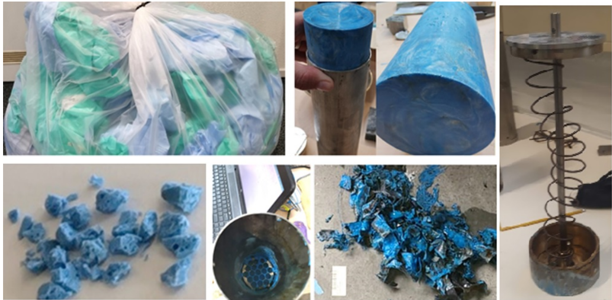
Figure 2.1: Overview of the remelting stages. From top left to bottom right: Collected WP waste, Melted WP into bars, Spring loaded system, Granulate, Filter in melting cylinder, Residue removed from filter and used for polluted dog-bones.
