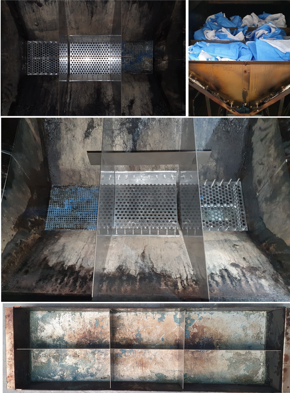
Figure 3.8: Test setup in the Sterimelt. Top left to bottom; Top view of loading bay with dividers, Loaded loading bay with clean WP waste and loading bay dividers, Side view of loading bay with dividers, End product tray with the tray divider used for testing.
