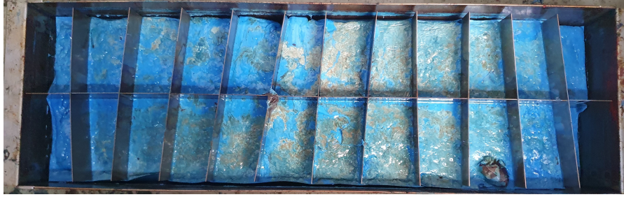
Figure 3.15: Tray with tray divider after a melting cycle.
