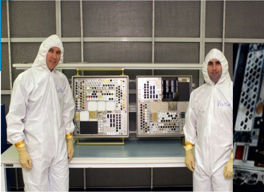
MISSE 3 Long duration space exposure test facility
