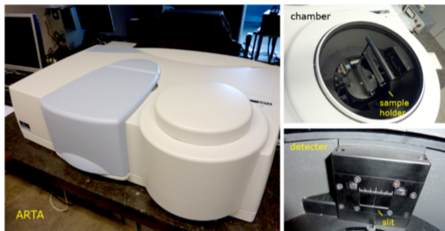
Figure 4.10 Photograph of the Automated Reflectance Transmittance Analyzer (ARTA) installed in the PerkinElmer Lambda 950 Spectrophotometer . From: Zhao, Enhancement of Light Trapping in Thin Film Silicon Solar Cells.
