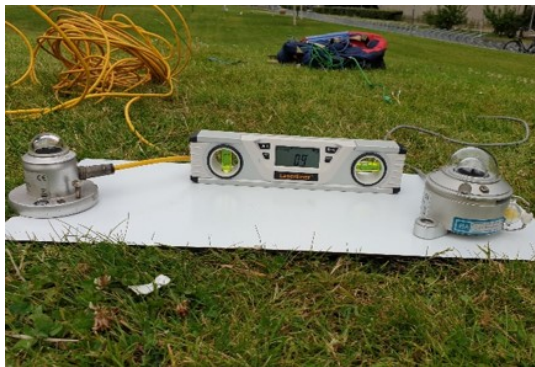
(a) The test was performed in a flat surface at zero tilt
