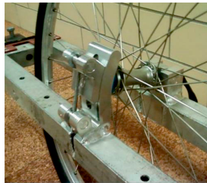
Figure 2.6 – Device to adjust the camber angle [93]. Starting from the first concept developed in [92] the authors added the possibility to adjust the camber angle.
