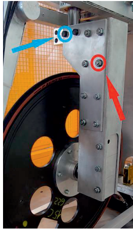
Figure 3.21 - Reinforcement of single-sided fork with 8 mm aluminium plate screws in the upper part (blue circle) and threaded bars (red circle).
