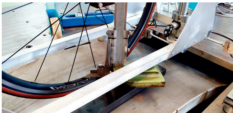
Figure 4.2 – Set-up for measuring the static tyre deflection with VeTyT, here depicted for RuotaVia drum.
