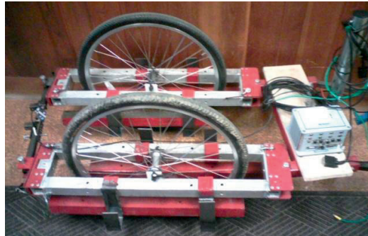
Figure 2.4 – Test device developed in [92]. A cart to be towed held two tyres, and a force sensor was placed in between the tyres to measure the lateral force.
