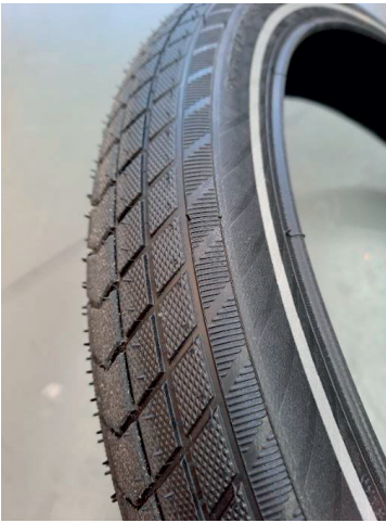
Figure 7.14 – Detail of tread pattern. In (A), Schwalbe Balloon (Big Ben Plus – T01) 20" x 2,15. In (B), CST Brooklyn (T02) 20" x 2,15.
