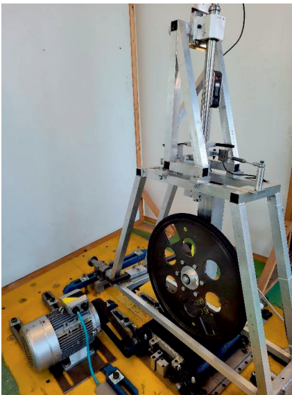
Figure 3.1 – First version of VeTyT test-rig. The frame resulted too deformable during the tests.
