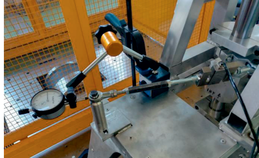
Figure 3.15 – Dial gauge used to measure the deflection of aluminium slender beam.
