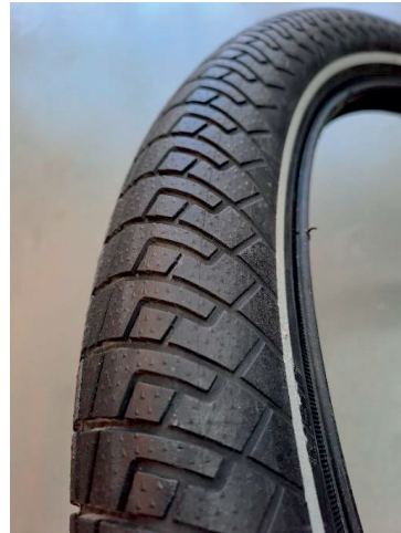
Figure 7.14 – Detail of tread pattern. In (A), Schwalbe Balloon (Big Ben Plus – T01) 20" x 2,15. In (B), CST Brooklyn (T02) 20" x 2,15.
