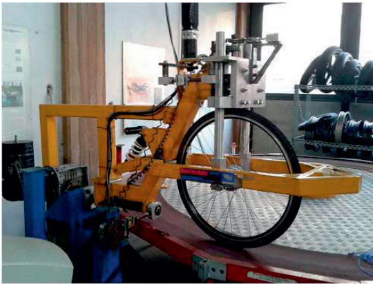
Figure 2.7 – Test-rig at University of Padua specifically configured for bicycle tyres [60]. Tyres were tested on a curved path, with different configurations of slip angle, camber angle and vertical loads.
