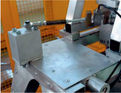
Figure 3.14 – New component with rectangular section, to replace the aluminium slender beam and ensure more stiffness.
