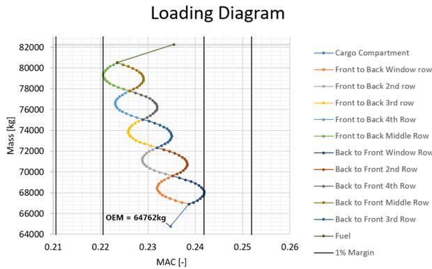
**Figure 9.2:** Loading diagram showing the position of the c.g. during loading of the Lightning2 aircraft.
