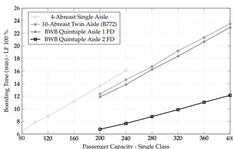
**Figure 15.1:** Boarding time of various aircraft as a function of passenger capacity (single class) [122].
