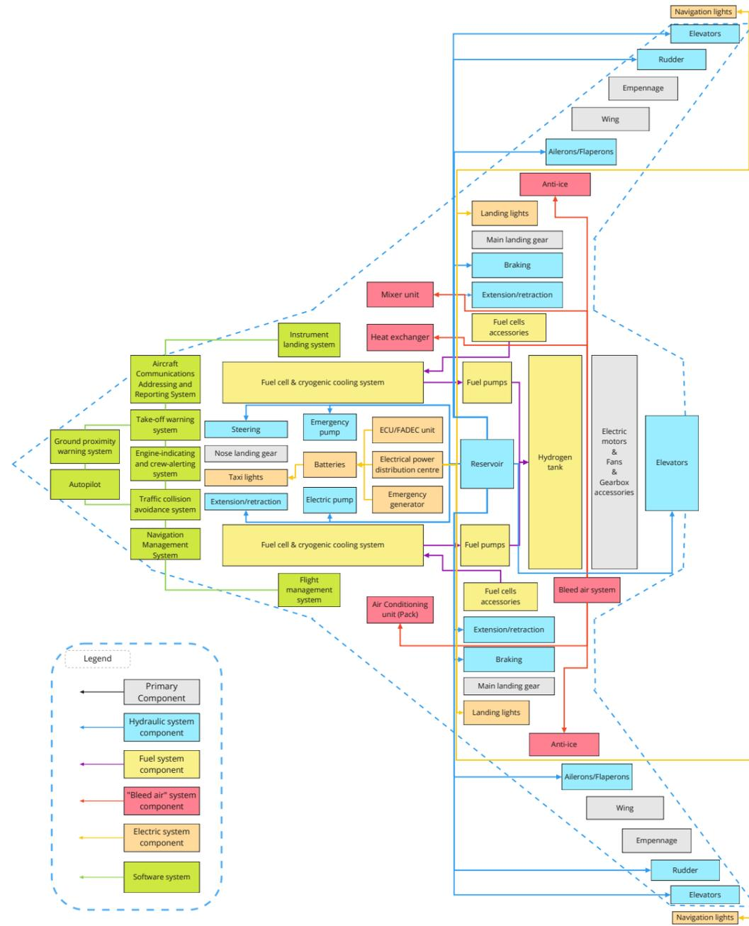
(a) Aircraft System Characteristics Diagram.
