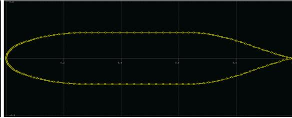
**Figure 7:** The custom airfoil used for the fuselage.
