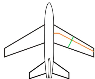
(b) *Swept wing elastic axis and cross-section.*
