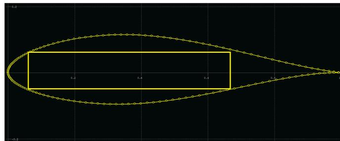
Figure 7.5: NACA 63<sub>4</sub> - 221 airfoil with cabin longitudinal cross-section fitted.
