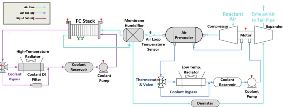
**Figure 6.3:** The fuel cell stack and balance of plant, including liquid cooling and air cooling systems [110].
