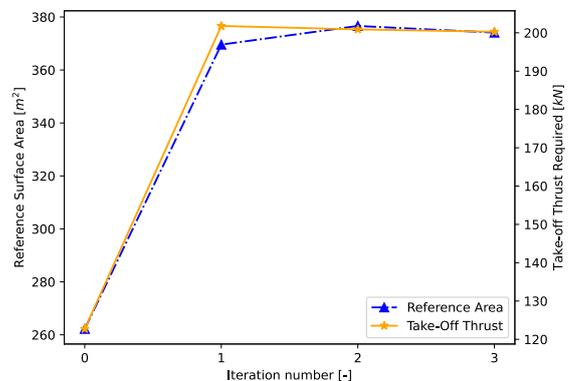
Figure 10.4: Change in reference surface area and take-off thrust required with iterations.
