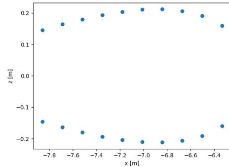
(b) Cross section example at span location of 15 metres in wingbox axis system after correction.
