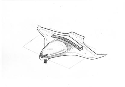
**Figure 3:** Drawing of the blended wing body wing concept.
