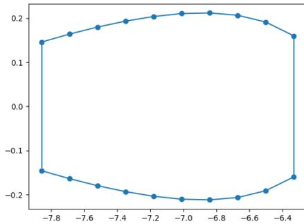
(a) Cross section example at span location of 15 metres in wingbox axis system before correction.
