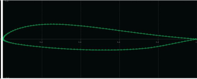
Figure 7.7: Eppler 325 airfoil.
