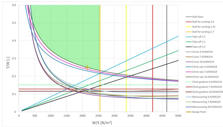
Figure 10.2: Iterated thrust and wing loading diagram indicating the feasible design space in green. The final design point is indicated by a plus.
