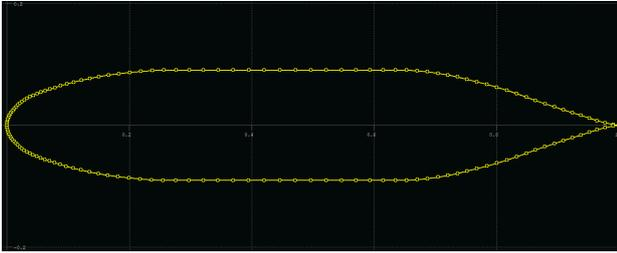
Figure 7.6: NACA 63<sub>4</sub> – 221 airfoil after modifications.
