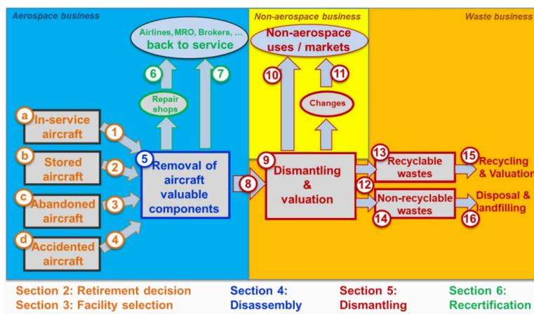
Figure 18.1: Process of aircraft decommissioning<sup>6</sup>.
