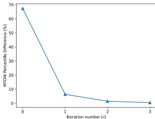
Figure 10.3: Percentage change in *MTOW* between iterations, showing the convergence of the iteration framework.
