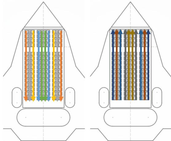
**Figure 9.3:** Two methods of loading passengers: front to back and back to front.
