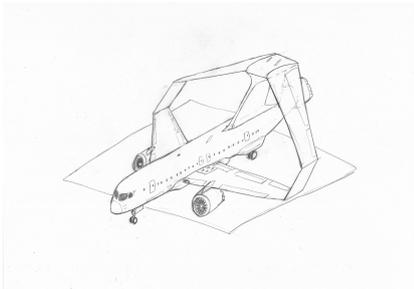
**Figure 2:** Drawing of the box wing concept.
