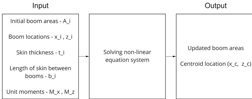
Figure 8.10: Flow diagram of boom area correction.
