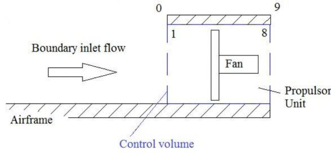
**Figure 6.1:** The simplified control volume of the ducted fan [68].
