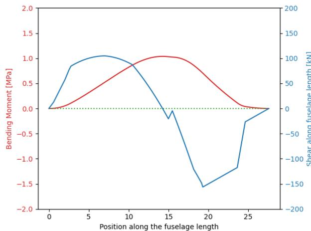
Figure 8.20: Shear and bending moment over the fuselage length.
