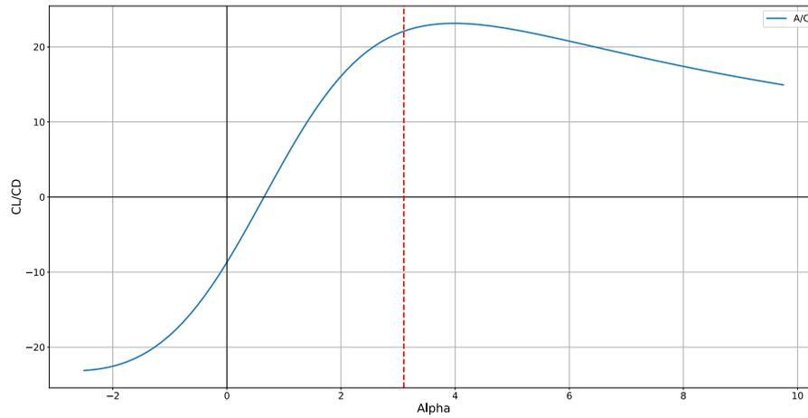
Figure 7.10:  $L/D$  ratio as a function of angle of attack.
