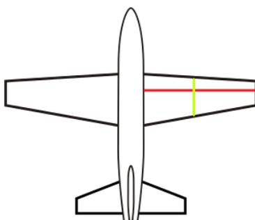
(a) *Un-swept wing elastic axis and cross-section.*
