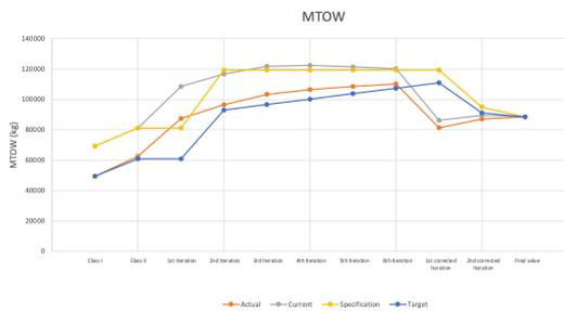
**Figure 11.1: Technical Performance Measurement for maximum take-off weight.**
