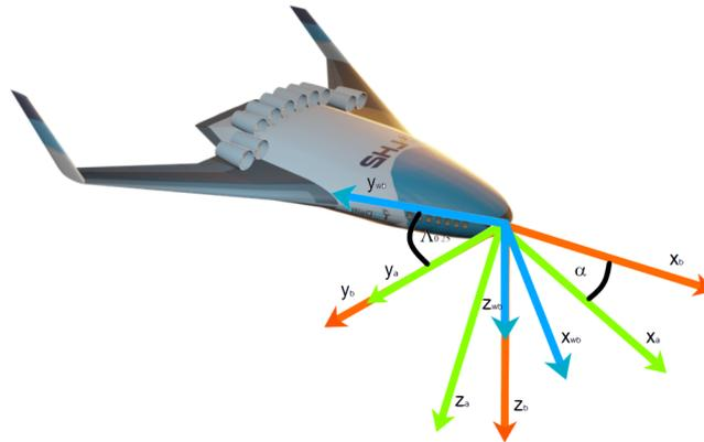
Figure 8.6: Three different axis system.
