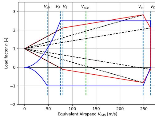
**Figure 8.4:** Manoeuvre and Gust Diagram for LC-7 and LC-8.
