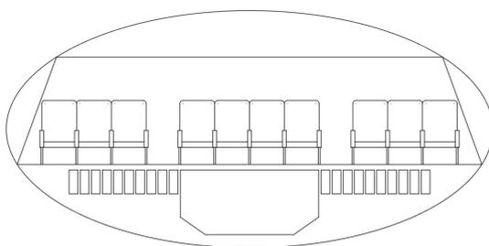
**Figure 19.1:** Fuselage cross section design.
