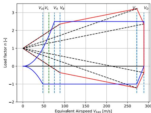
**Figure 8.2:** Manoeuvre and Gust Diagram for LC-3 and LC-4.
