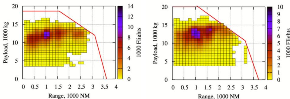
**Figure 2.4:** Heat maps of payload-range diagram of the A320 (left) and the B737 (right) [65].
