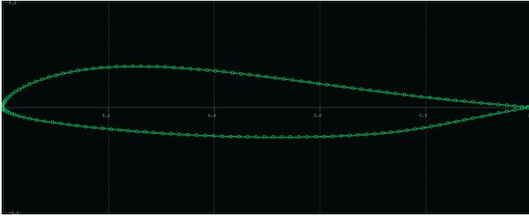
**Figure 6:** The Eppler 325 airfoil used for the wing.
