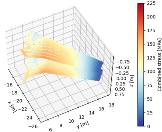
**Figure 8:** Complete stress distribution of wingbox from side view.
