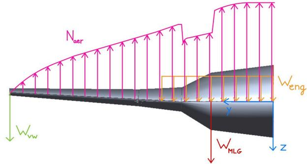
**Figure 8.8:** The free body diagram for half of the aircraft viewed from the front.
