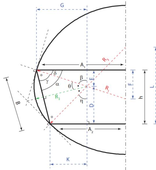
Figure 8.19: Oval fuselage dimensions [99].
