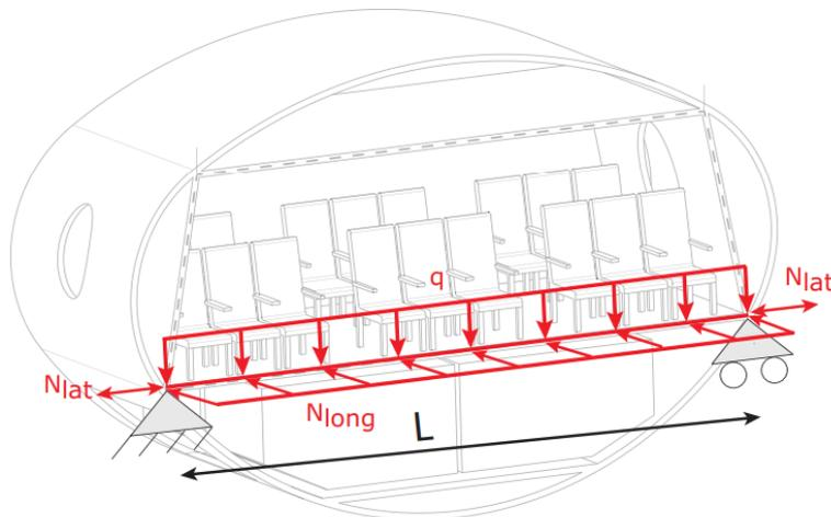
Figure 8.23: Visual representation of floor loading [99].
