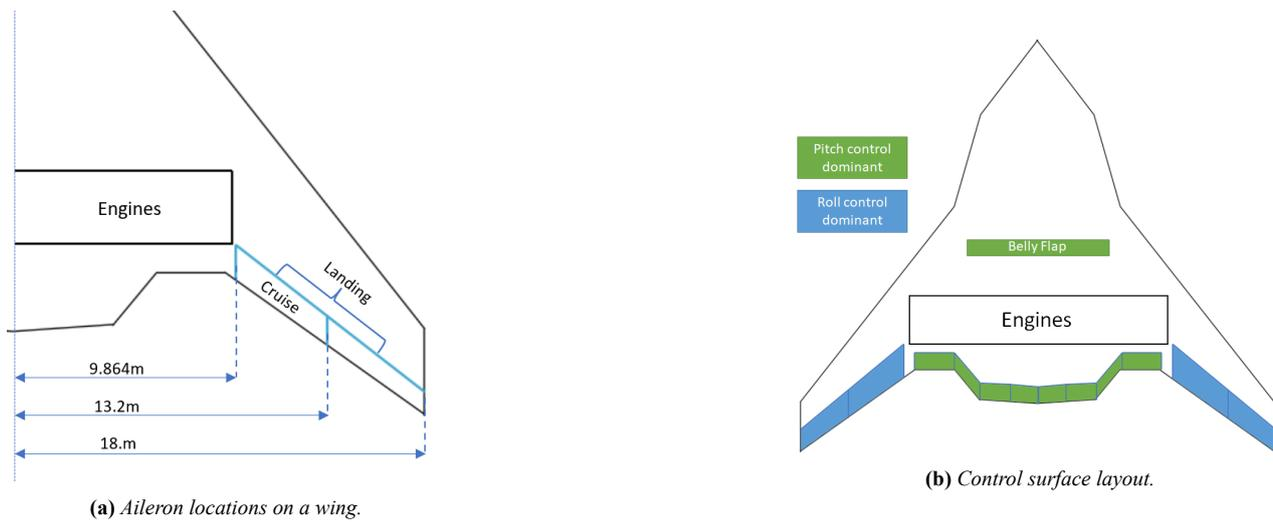
Figure 9.4: Placement of control surfaces on the Lightning2 aircraft.
