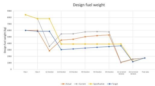
**Figure 11.2: Technical Performance Measurement for design fuel weight.**
