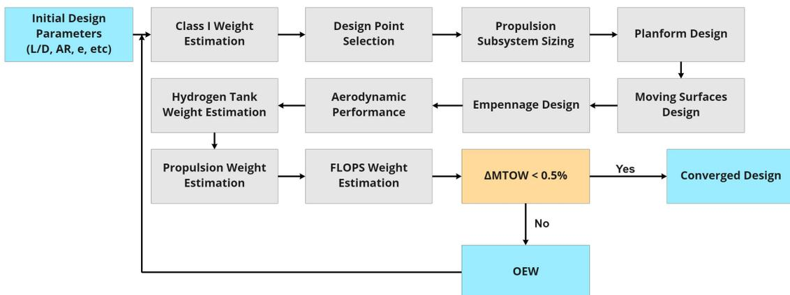
Figure 10.1: Flow diagram of the iteration framework.
