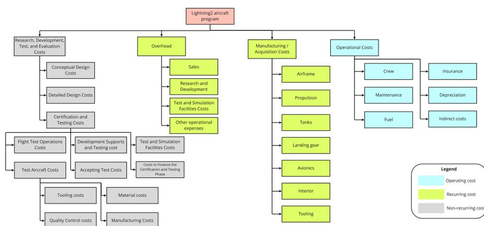
Figure 3.1: Cost breakdown structure for the Lightning2 aircraft.
