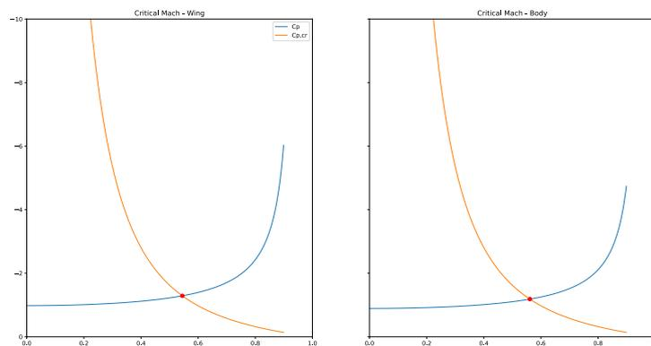
Figure 7.11: Critical pressure coefficients, wing and body.
