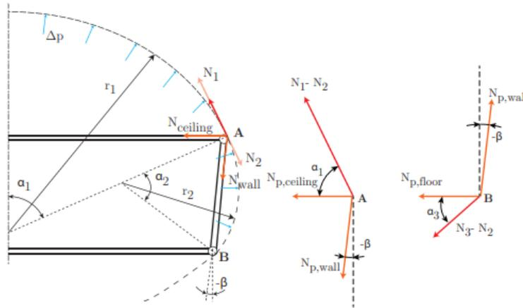
Figure 8.21: Node analysis for the oval fuselage [99].
