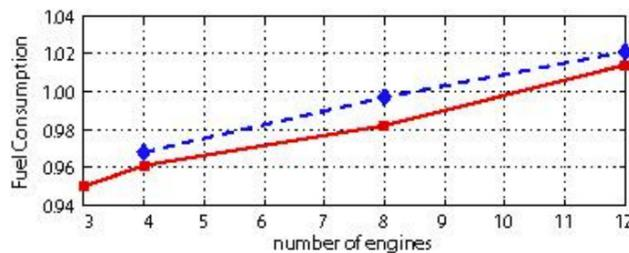
Figure 6.2: Fuel consumption with BLI for varying number of engines [57].
