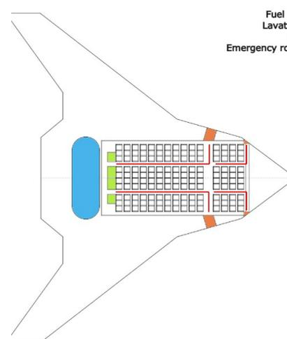
**Figure 19.2:** Fuselage top view layout.
