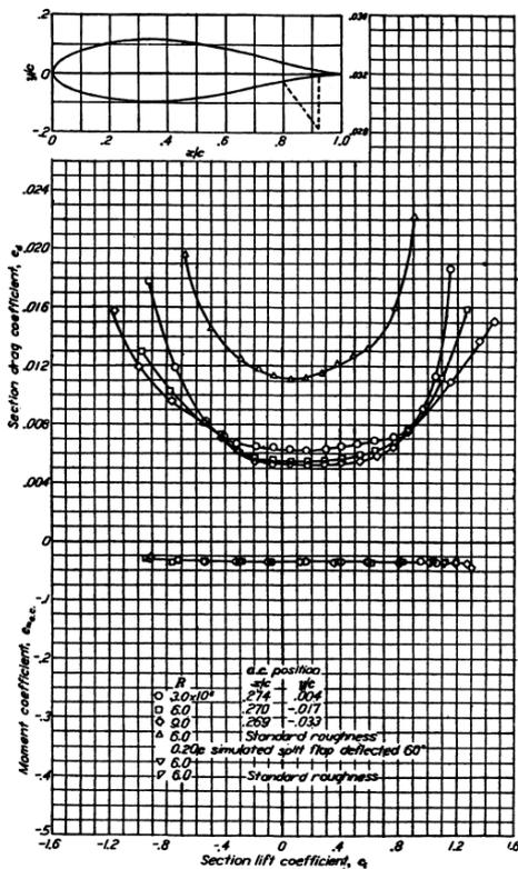
Figure 7.4: Experimental plots of the NACA 63<sub>4</sub> - 221 airfoil.[3]
