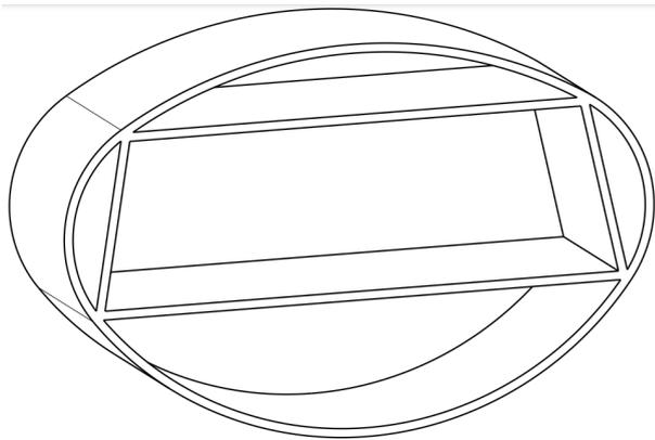
Figure 8.18: Oval fuselage layout [99].
