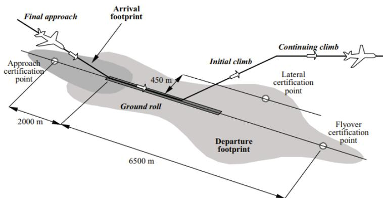
**Figure 12.1:** Noise footprint definitions for approach, fly-over, and lateral certification points [33].
