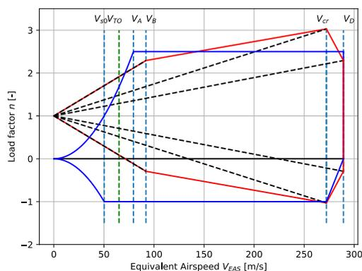
**Figure 8.1:** Manoeuvre and Gust Diagram for LC-1 and LC-2.
