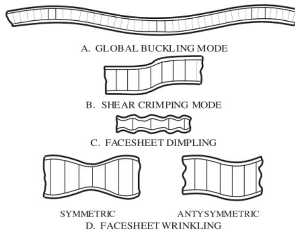
**Figure 8.25:** Failure modes of a sandwich panel [52].
