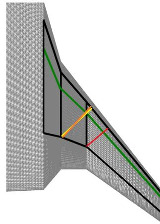
Figure 8.16: Top view of wingbox structure in which the black line indicates the outline of structure and green line indicates the elastic axis.
