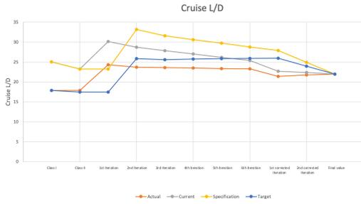
Figure 11.3: Technical Performance Measurement for cruise L/D.
