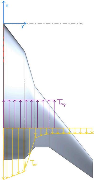
**Figure 8.7:** The free body diagram for half of the aircraft viewed from the top.
