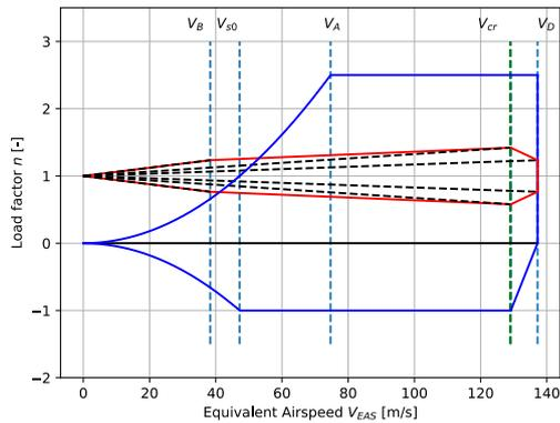
**Figure 8.3:** Manoeuvre and Gust Diagram for LC-5 and LC-6.
