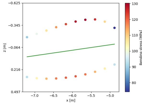
Figure 8.12: Bending stress distribution at an arbitrary span location in wingbox coordinate system.
