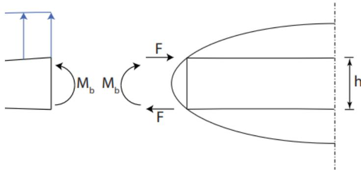
Figure 8.22: Example wing bending for positive load factors.
