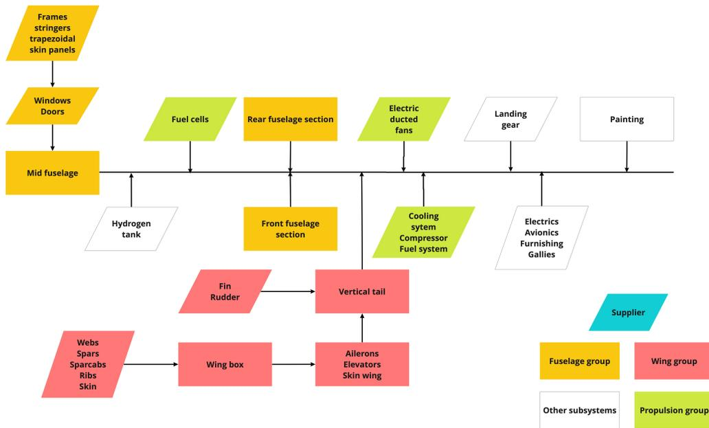
Figure 17.1: Assembly line for Lightning2.
