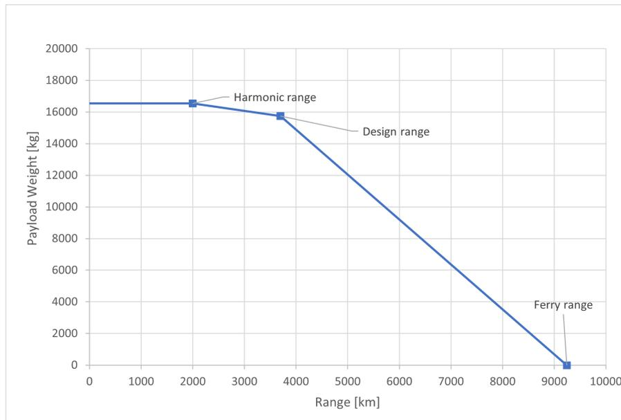
Figure 10.5: Payload-range diagram for the iterated final design of the Lightning2 aircraft.
