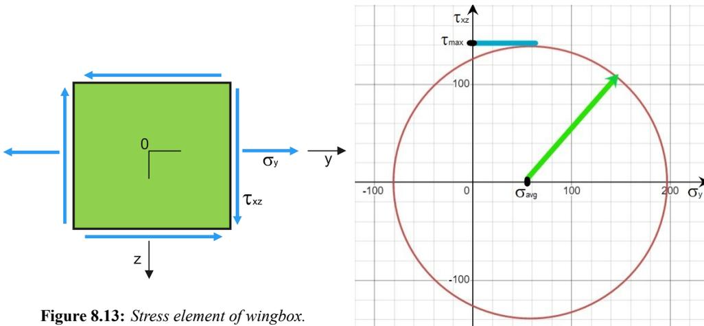
Figure 8.13: Stress element of wingbox.
