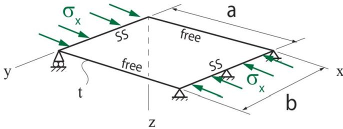
Figure 8.24: Clean thin sheet buckling free body diagram [26].
