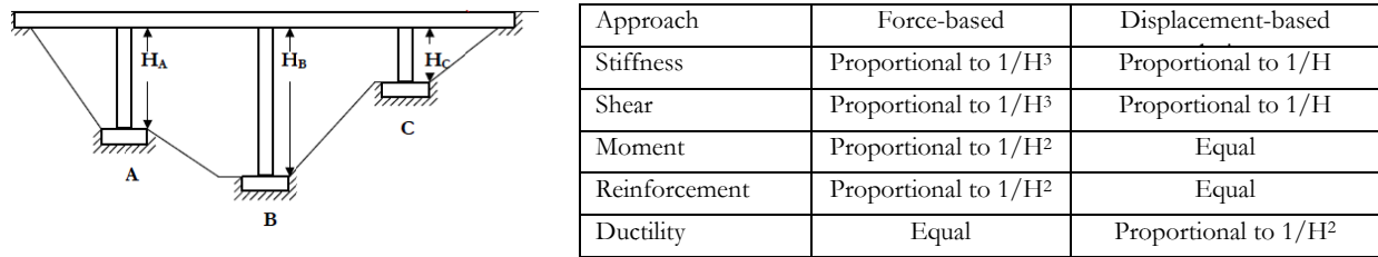
Figure 19 - Implications of using different approaches. Example extracted from the work of Lourenco P.
