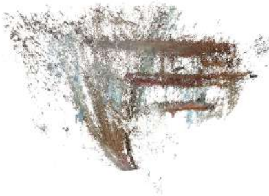
Figure 5.2: Point cloud extracted based on 159 video frames while filming for 28 seconds. Room: Hallway Geolab in the Architecture building. Software used: Pix4D with the standard setting 3D Models .
