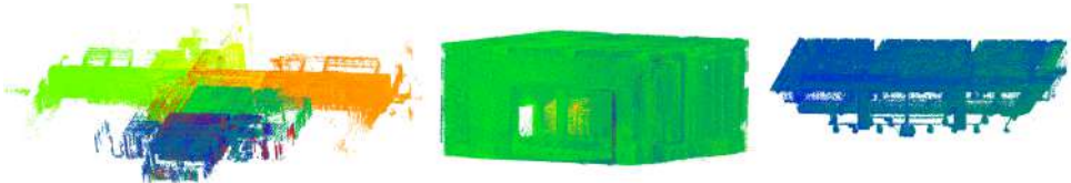
Figure 5.13: Example of the results of manual wall points removal. From left to right: a full point cloud measurement, clipping rooms as separate subsets and then extracting the ceiling without wall points.
