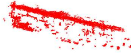
Figure 7.8: Screen shot of the point cloud displaying the hallway near the entrance of Berlage hall from DIM. The point cloud is down sampled using the additionally suggested noise removal.
