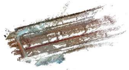
Figure 5.3: Point cloud extracted based on 159 video frames while filming for 28 seconds. Room: Hallway Geolab in the Architecture building. Software used: Pix4D with the standard setting 3D Maps .
