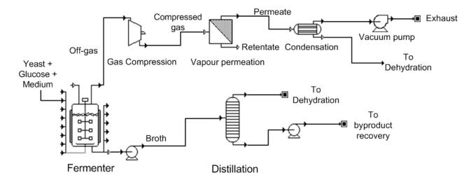
Ethanol recovery from fermentation off–gas by vapour permeation with recovered ethanol fed to distillation.
