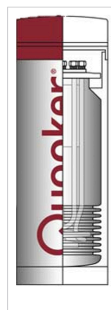
Figure 75. Bellow reservoir within Quooker, expands when water is heated up and retracts upon valve opening
