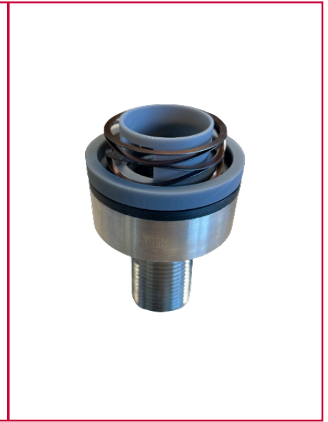
9. The wave spring is placed in the groove.
