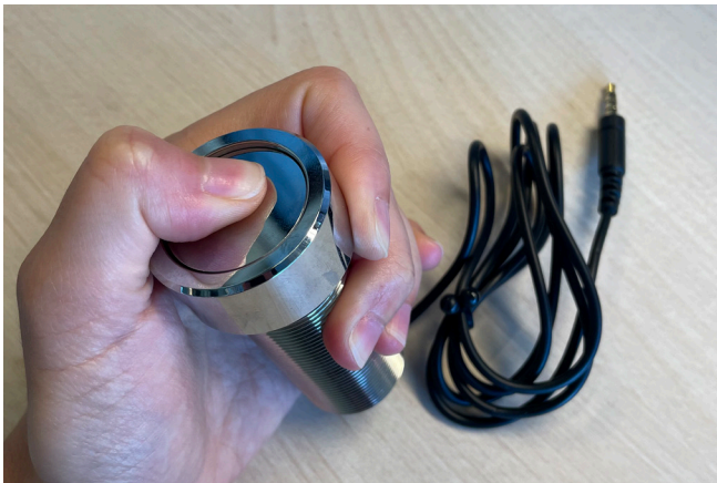
Figure 34. a) Wizard of Oz prototype with hidden electronics b) Wired button to control the tap
