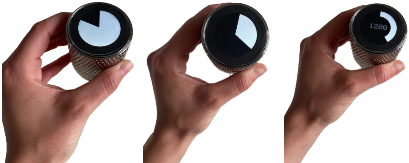
Figure 76. a) Rotating to set volume b) Pushing for preset c) Push and wait to switch modes
