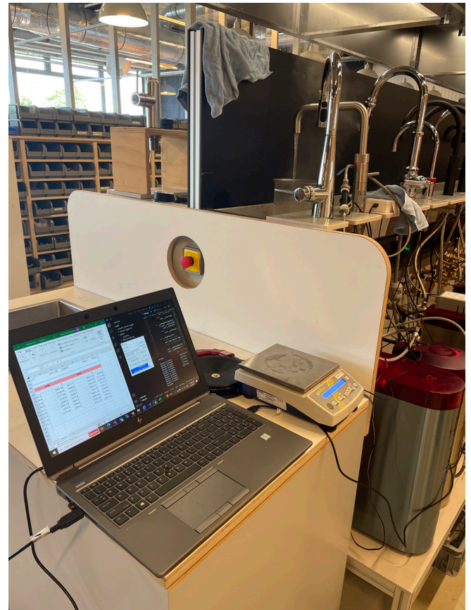
Figure 70. Flow Sensor Test Set-up; Quooker system, flow sensor, laptop with control application, container, precision scale
