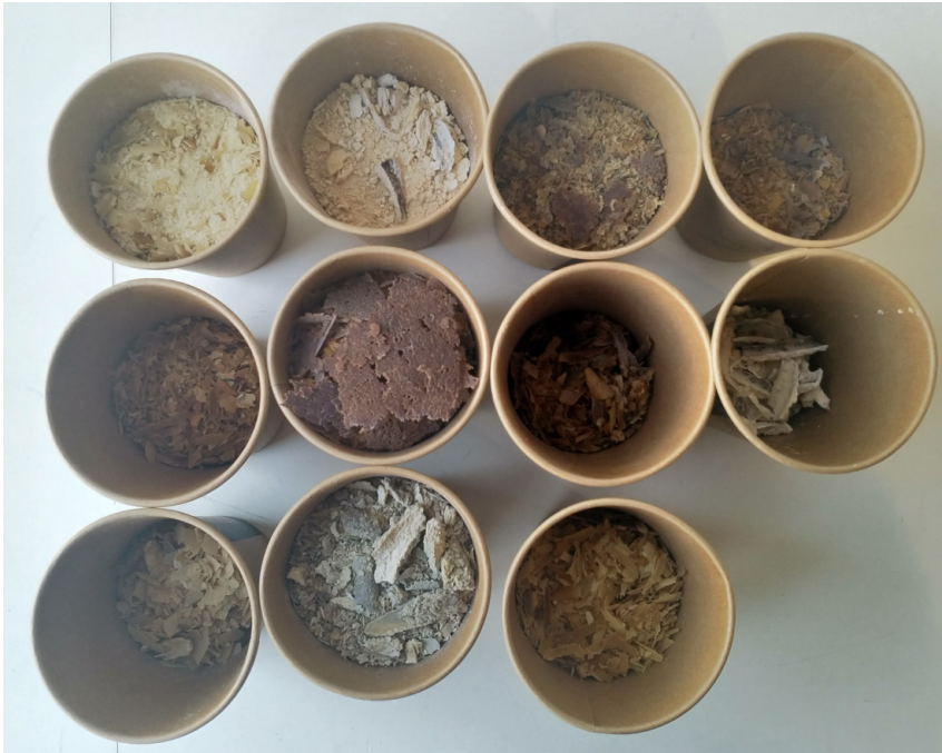
Figure 61. Limescale Buildup collected from Quooker reservoirs in different countries.
