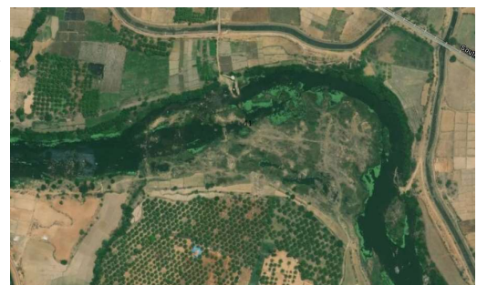
Fig. 5.8 Terrestrialization of river bed downstream of a dam in Kaveri basin (Source: ESRI Digital Globe Imagery)
