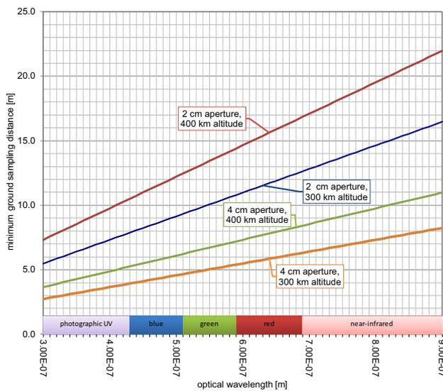
**Fig. 10** Ground sampling distance of diffraction limited cameras
