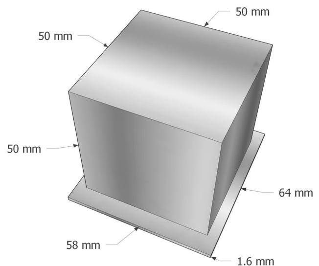
**Fig. 2** 1p PocketQube with body mounted solar cells
