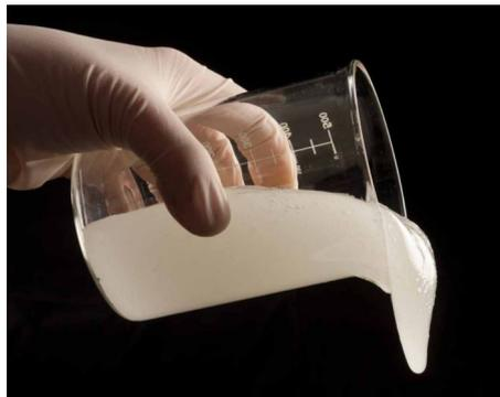
Figure 1.1: Visco-elastic diverting acid. [9]
