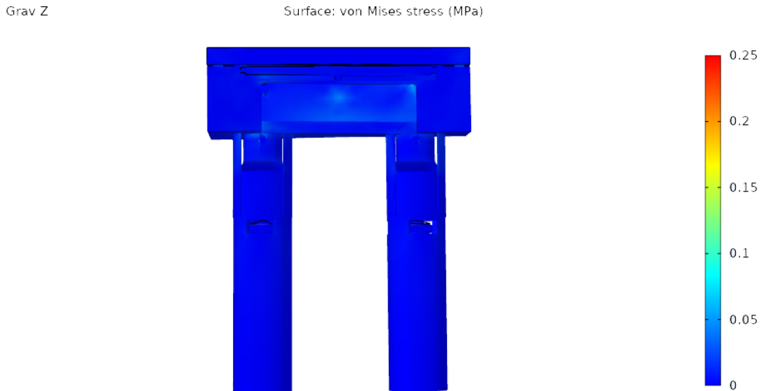
Figure 6.24: Deformation of the Gravity Release in Z axis
