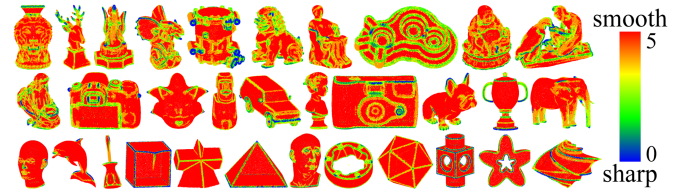
Fig. 5. Geometric feature levels (0-5) of each point in the training dataset. The lower geometric feature levels (in blue) represent sharper regions.
