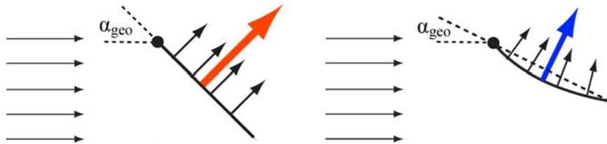
**Fig. 8** Net force angle as a function of geometric angle of attack *Left*: Rigid wing. *Right*: Flexible wing. Apparent reference flow from left-to-right. Small vectors represent local net forces that act normal to the wing surface, and big vector represent resultant net force that is aligned with respect to the geometric angle of attack.
