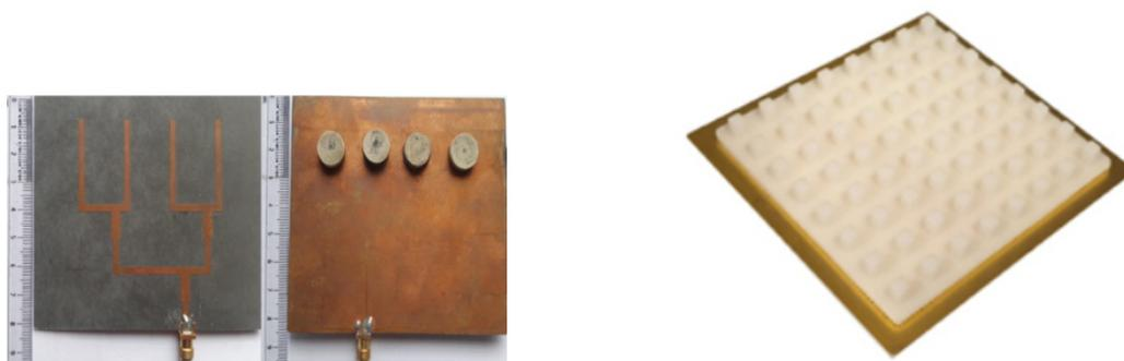
**Figure 1.1:** Dielectric Resonator Antennas [3, 4]
