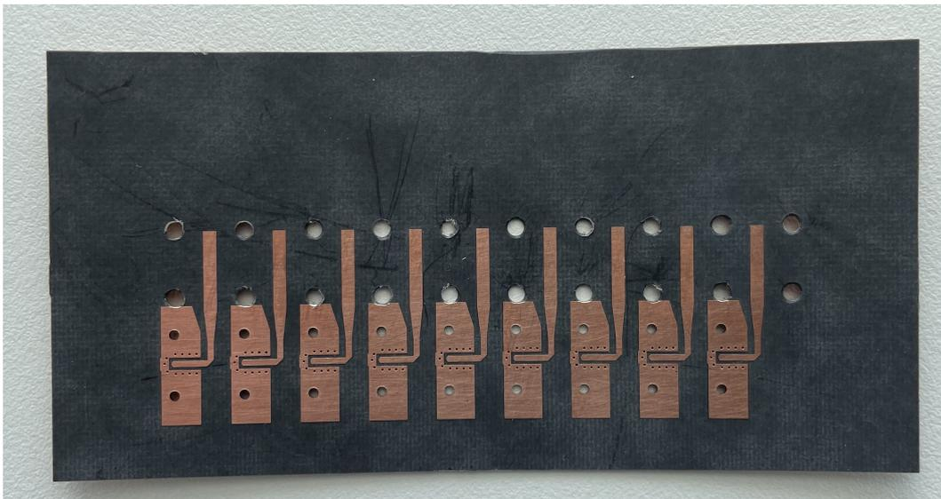
**Figure 6.4:** Feed network for array (bottom)
