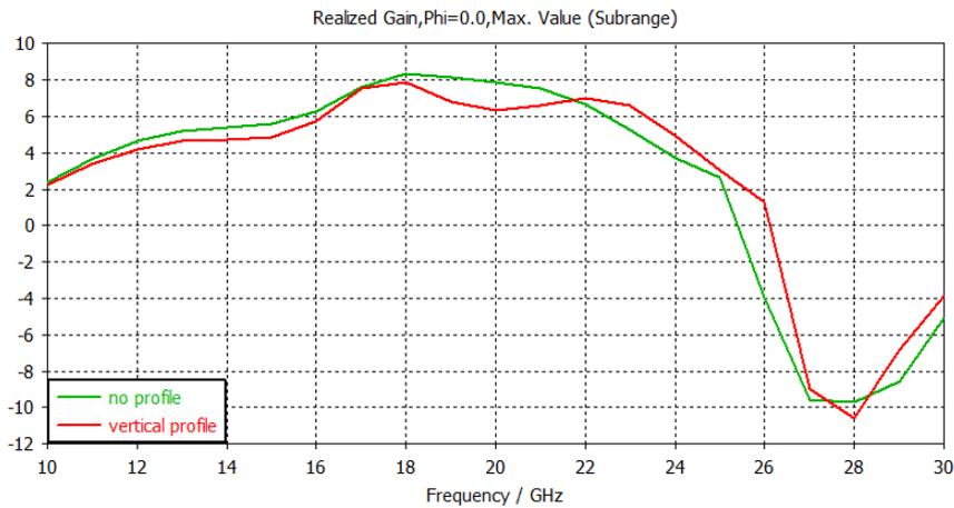
Figure 5.35: Gain vs Frequency comparison (profile 1 vs homogeneous permittivity, single element, slot fed)
