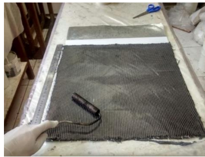
Fig. 1 Carbon fiber lamination process
