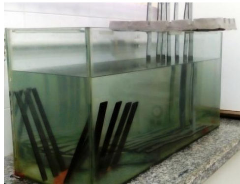
32 Fig. 3 Specimens in salt water tank
