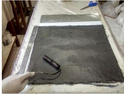
Fig. 1 Carbon fiber lamination process
