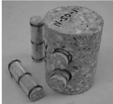
Figure 3.6 NMR samples wrapped in plastic and placed back into the cylindrical specimen.
