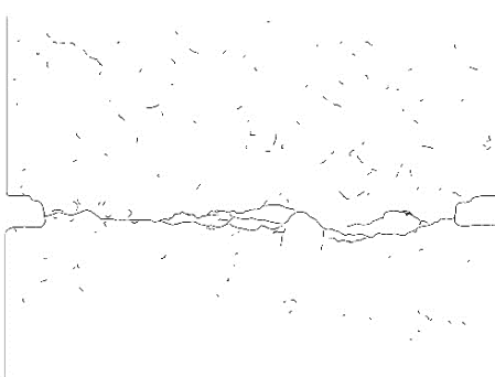
Figure 5.37 Fracture pattern for representative static test on BFS cement concrete Wet (26c7).
