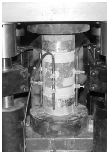
Figure 3.8 Detail of static specimen glued into set-up.
