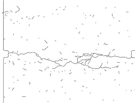
Figure 5.40 Fracture pattern for representative MSHB test on BFS cement concrete Wet (07HW04).
