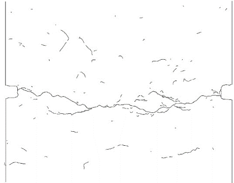
Figure 5.33 Fracture pattern for representative MSHB test on Portland cement concrete Dry (D02).
