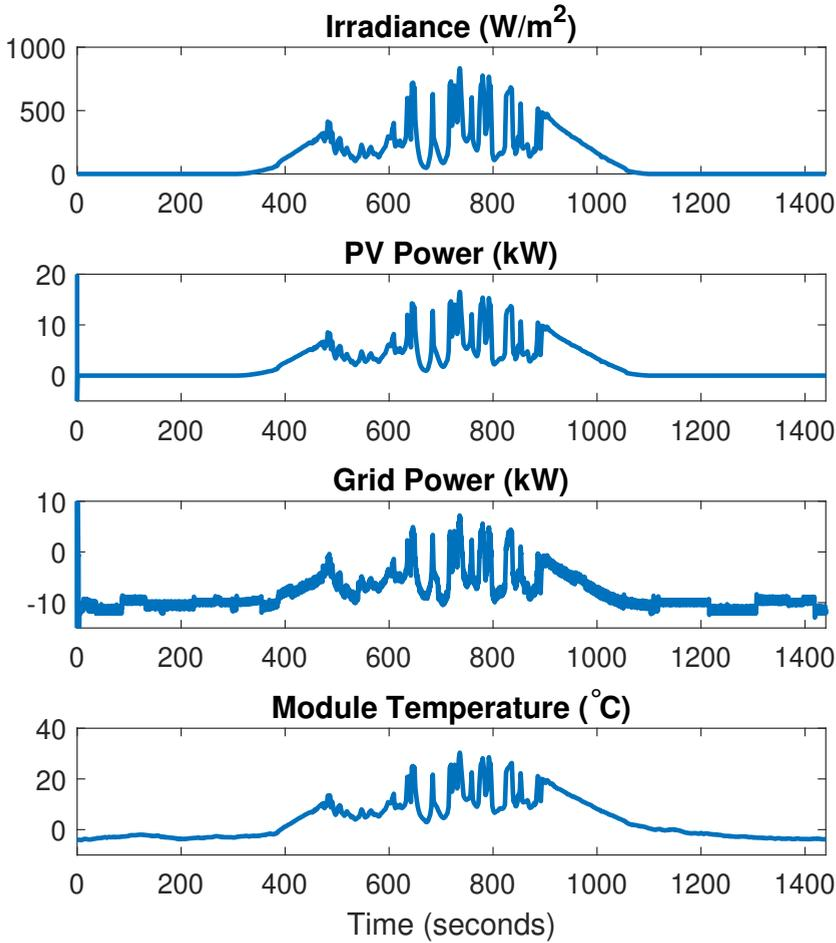
Figure 5.21: Irradiance, PV Power, Import/Export of Grid Power and Module Temperature on a day with highly varying ambient conditions
