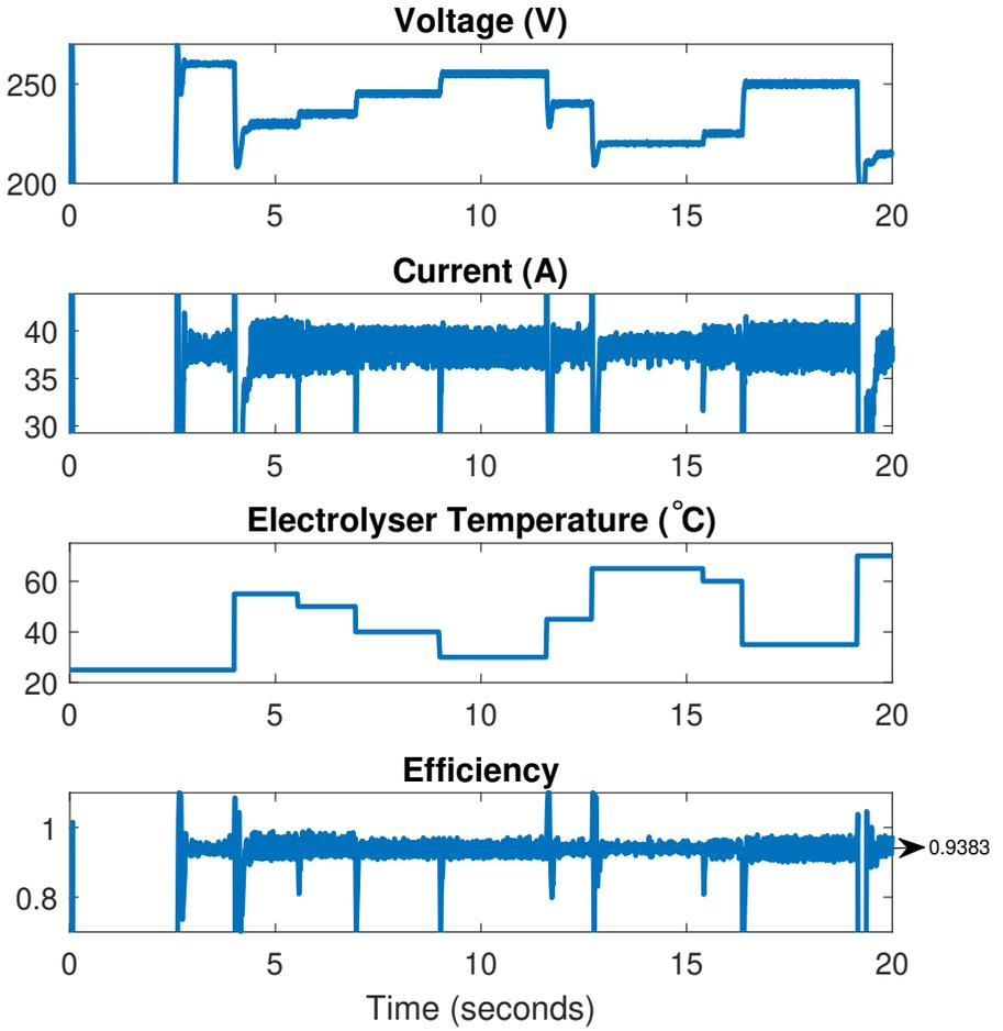
Figure 5.14: Voltage, Current, Electrolyser Temperature and Efficiency with varying electrolyser temperature, constant irradiance and varying module temperature
