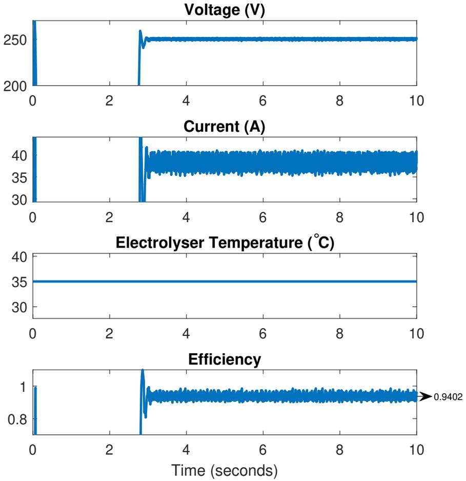
Figure 5.4: Voltage, Current, Electrolyser Temperature and Efficiency when the temperature of the electrolyser is constant at 35°C
