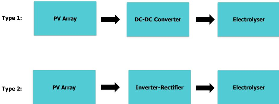
Figure 2.2: Different possible power electronic interfaces between the PV array and the electrolyser
