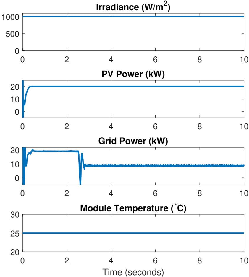
Figure 5.1: Irradiance, PV Power, Import/Export of Grid Power and Module Temperature when the temperature of the electrolyser is constant at 25°C
