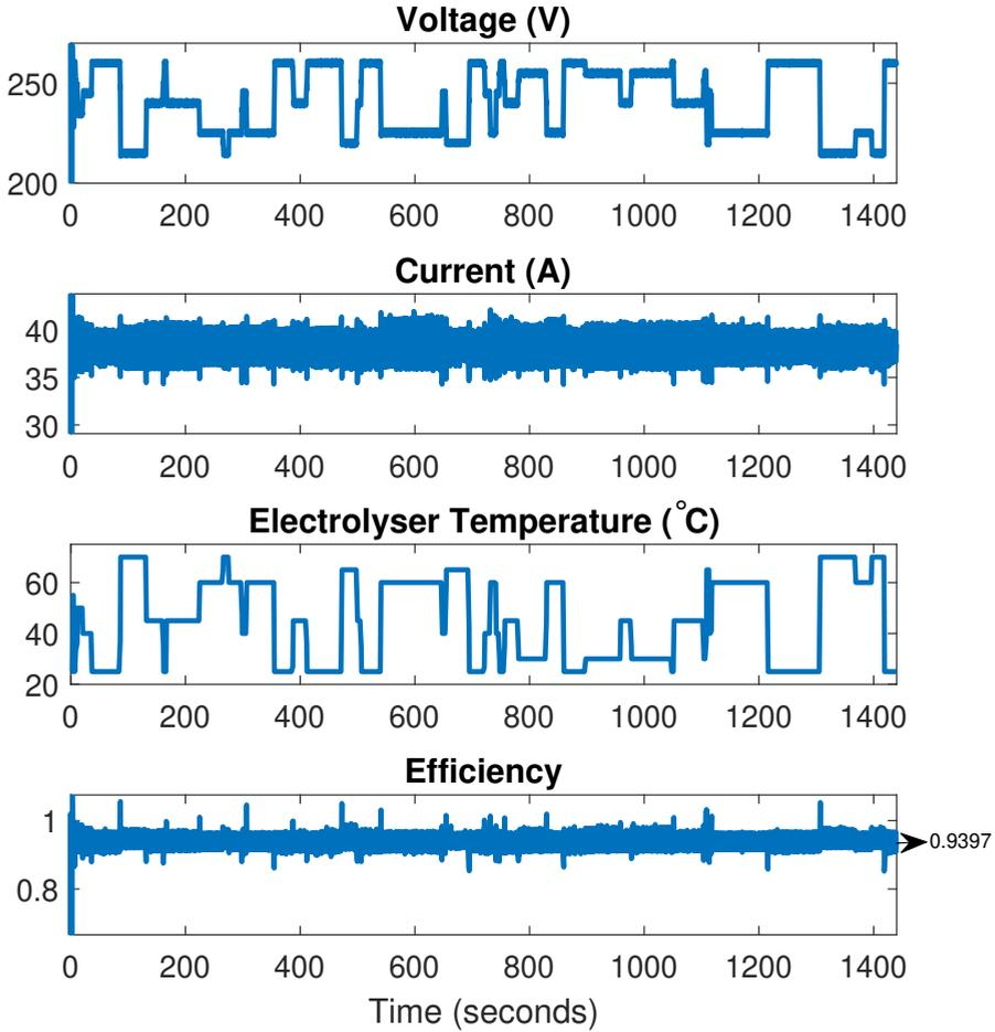
Figure 5.20: Voltage, Current, Electrolyser Temperature and Efficiency on a clear day
