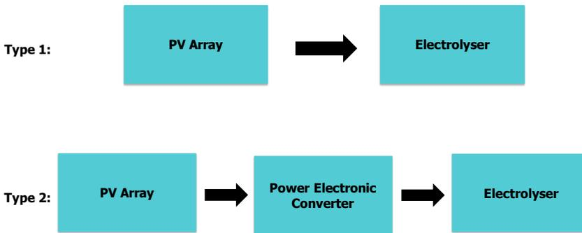
Figure 2.1: Topologies with and without a power electronic interface between the PV array and the electrolyser
