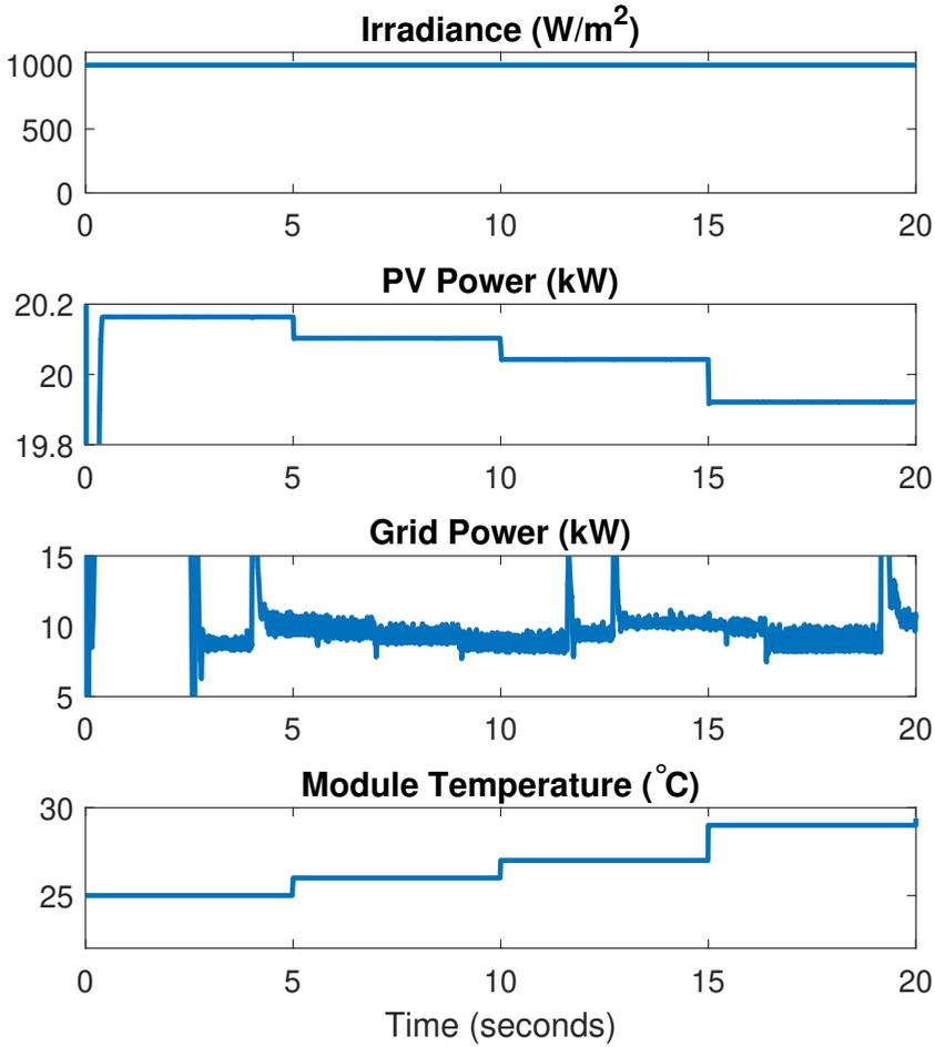
Figure 5.13: Irradiance, PV Power, Import/Export of Grid Power and Module Temperature with varying electrolyser temperature, constant irradiance and varying module temperature
