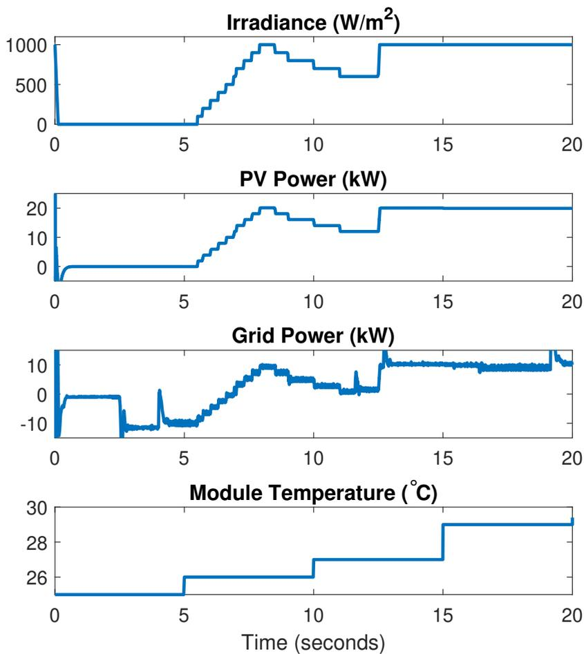
Figure 5.15: Irradiance, PV Power, Import/Export of Grid Power and Module Temperature with varying electrolyser temperature, varying irradiance and varying module temperature
