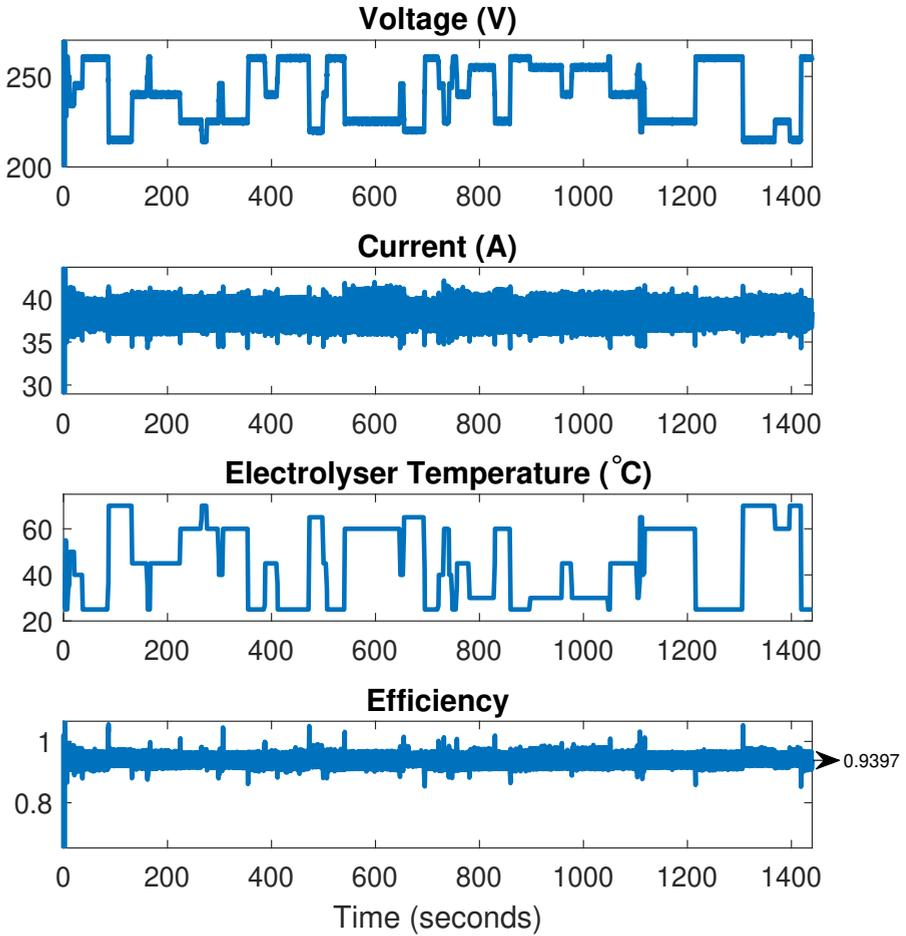
Figure 5.22: Voltage, Current, Electrolyser Temperature and Efficiency on a day with highly varying ambient conditions
