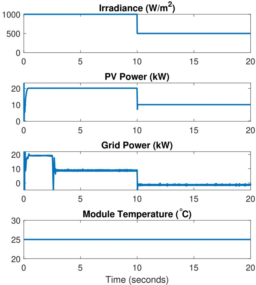
Figure 5.11: Irradiance, PV Power, Import/Export of Grid Power and Module Temperature with constant electrolyser temperature, varying irradiance and constant module temperature
