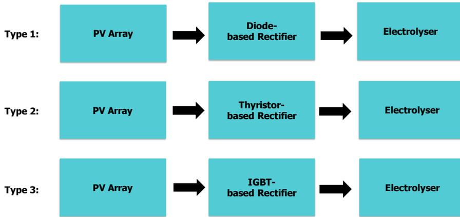
Figure 2.3: Different types of rectifiers which could be employed in the system
