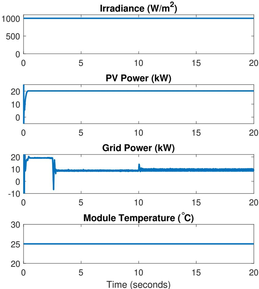
Figure 5.5: Irradiance, PV Power, Import/Export of Grid Power and Module Temperature when the temperature of the electrolyser changes from 25°C to 35°C
