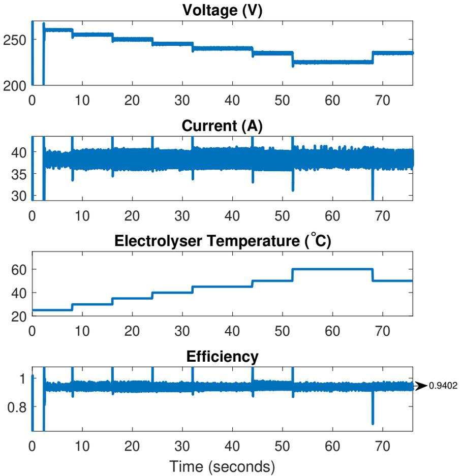
Figure 5.18: Voltage, Current, Electrolyser Temperature and Efficiency with varying electrolyser temperature, varying irradiance and varying module temperature
