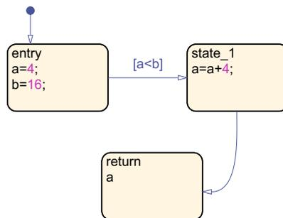
Figure A.1: A Stateflow Chart containing a simple function
