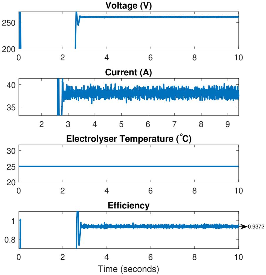
Figure 5.2: Voltage, Current, Electrolyser Temperature and Efficiency when the temperature of the electrolyser is constant at 25°C
