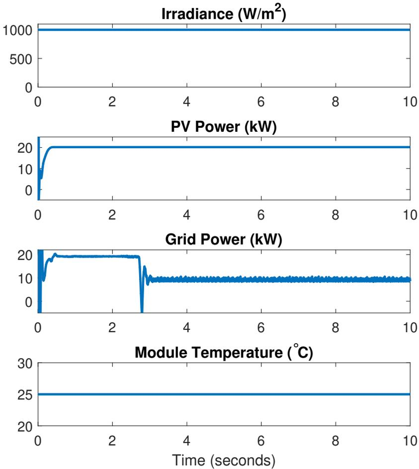
Figure 5.3: Irradiance, PV Power, Import/Export of Grid Power and Module Temperature when the temperature of the electrolyser is constant at 35°C
