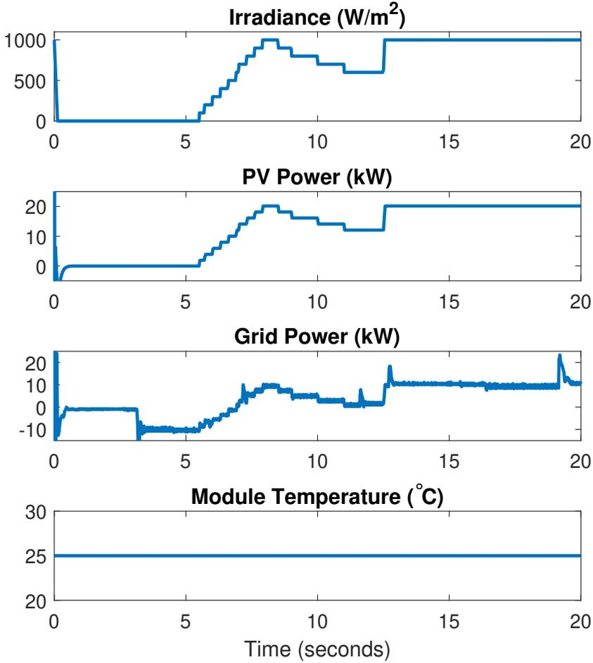
Figure 5.9: Irradiance, PV Power, Import/Export of Grid Power and Module Temperature with varying electrolyser temperature, varying irradiance and constant module temperature
