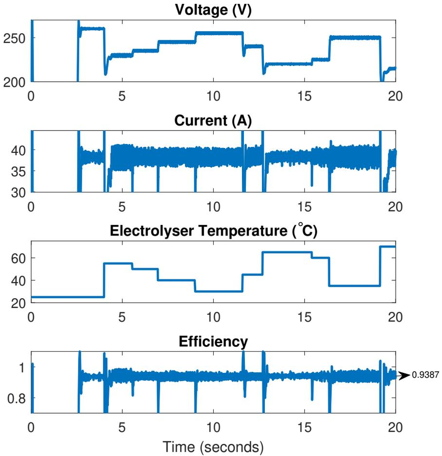
Figure 5.16: Voltage, Current, Electrolyser Temperature and Efficiency with varying electrolyser temperature, varying irradiance and varying module temperature
