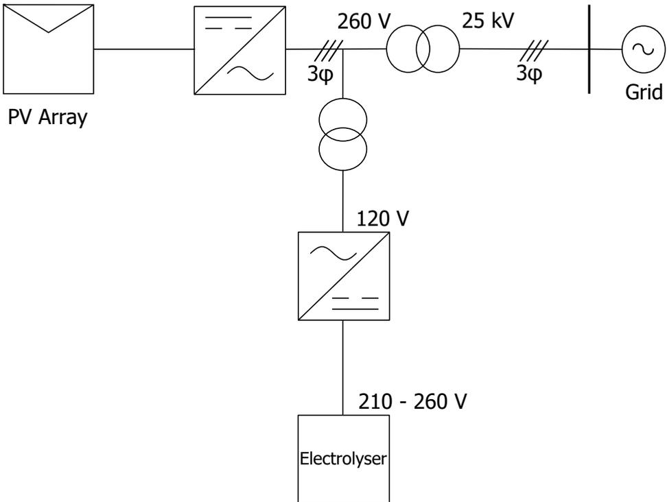
Figure 3.4: A single line diagram of the system
