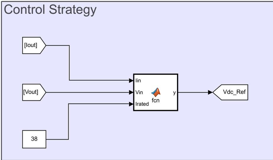
Figure 4.4: The control strategy's MATLAB Function Block in the Simulink model
