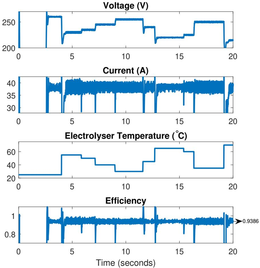
Figure 5.8: Voltage, Current, Electrolyser Temperature and Efficiency when the temperature of the electrolyser ranges from 25°C to 70°C
