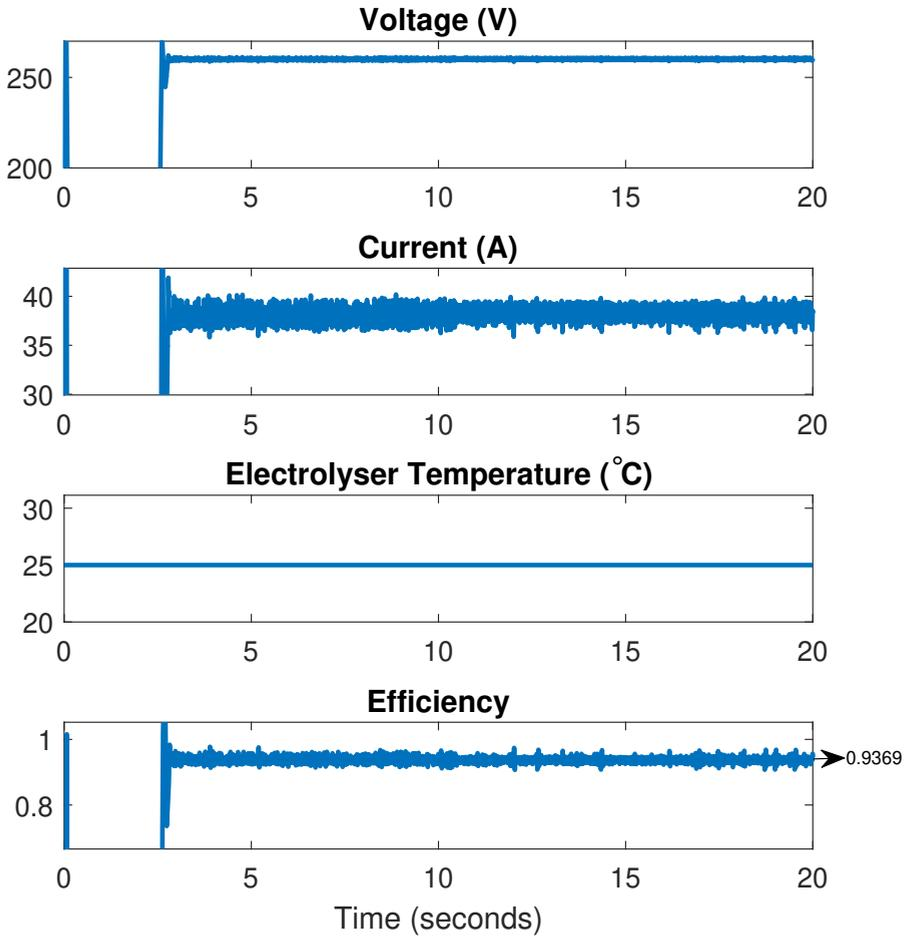
Figure 5.12: Voltage, Current, Electrolyser Temperature and Efficiency with constant electrolyser temperature, varying irradiance and constant module temperature
