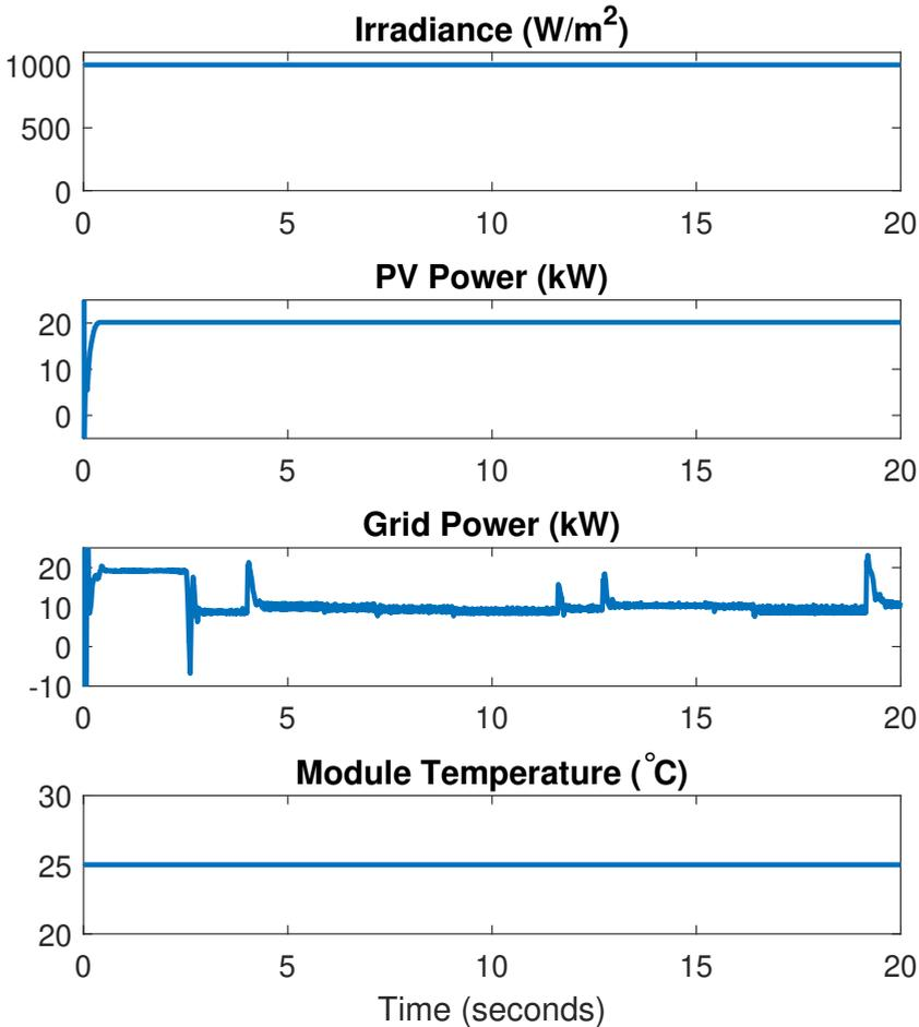
Figure 5.7: Irradiance, PV Power, Import/Export of Grid Power and Module Temperature when the temperature of the electrolyser ranges from 25°C to 70°C
