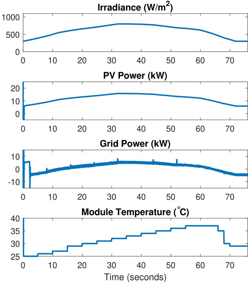
Figure 5.17: Irradiance, PV Power, Import/Export of Grid Power and Module Temperature with varying electrolyser temperature, varying irradiance and varying module temperature
