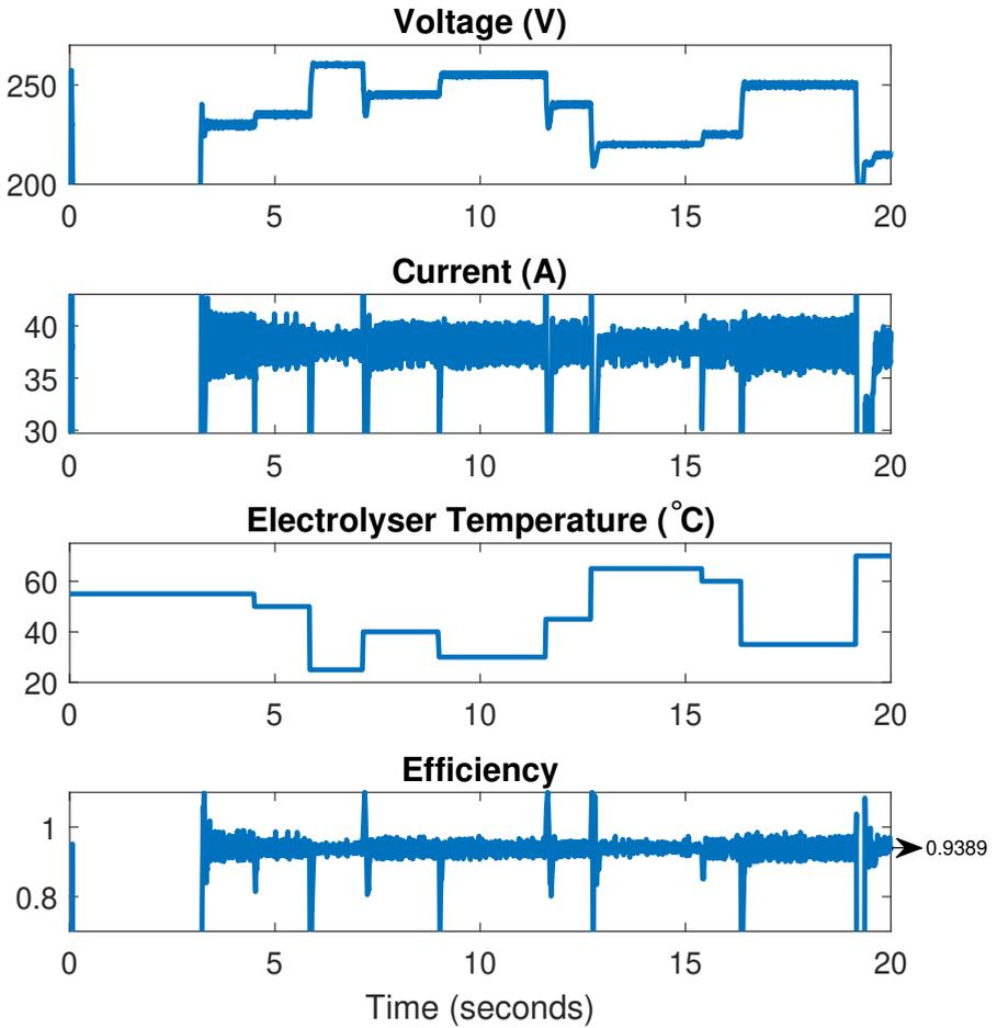
Figure 5.10: Voltage, Current, Electrolyser Temperature and Efficiency with varying electrolyser temperature, varying irradiance and constant module temperature
