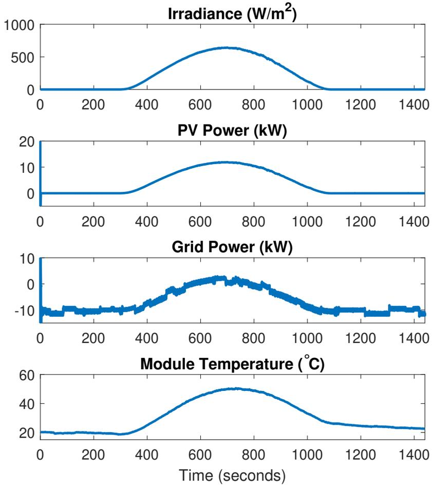
Figure 5.19: Irradiance, PV Power, Import/Export of Grid Power and Module Temperature on a clear day
