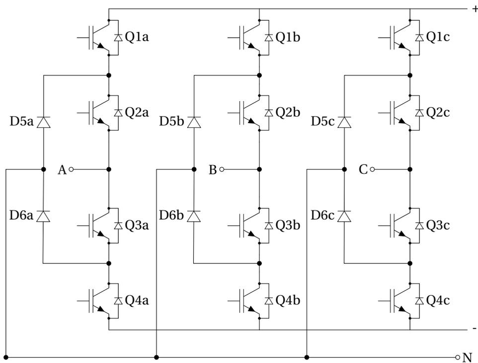
Figure 2.4: Three Level Converter
