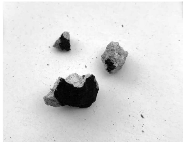
Figure 10 – Produced meteorite fragments after the artificial main body hit a hard underground.
