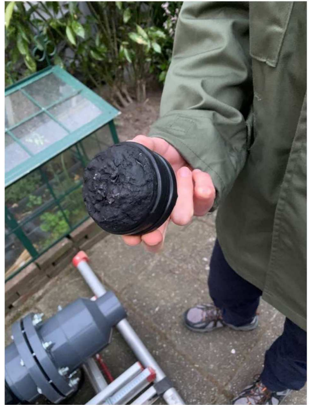
Figure 9 – Example of an artificial meteorite, made of concrete, mass ~250 g.
