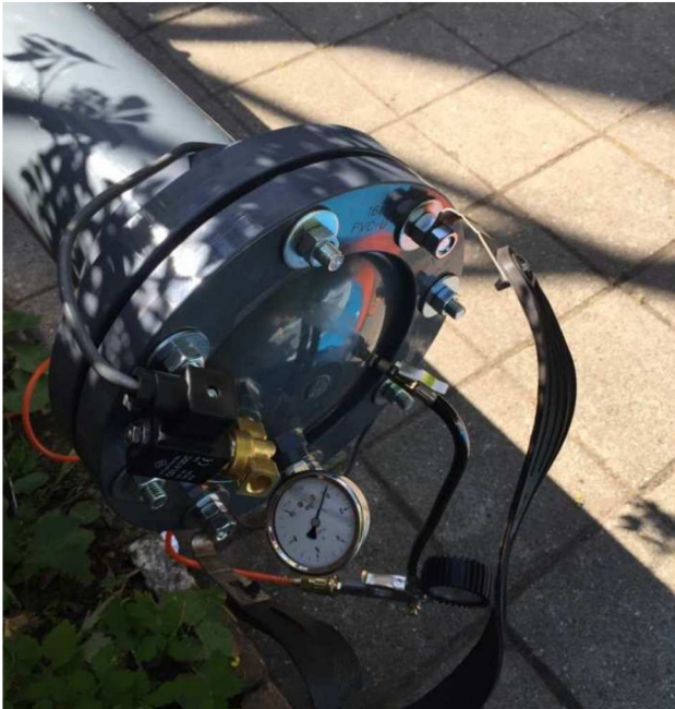
Figure 6 – Backside of the apparatus with manometer, release valve and filling valve.
