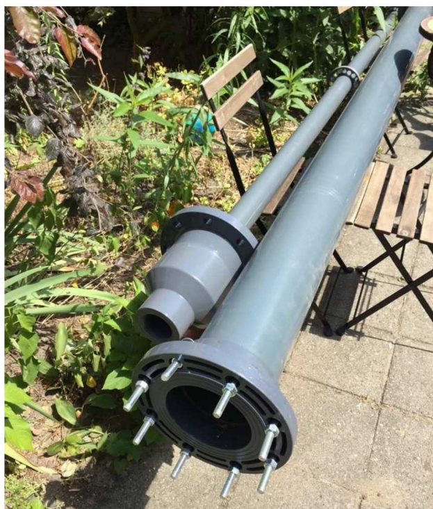
Figure 5 – Construction of the apparatus. The inner tube is the actual launch tube, which will be mounted into the large one, which acts as the reservoir with compressed air.
