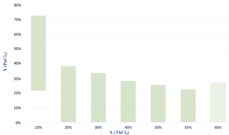
Fig. 8. Chart of the maximal safe molar concentration* of \text{PuCl}_3 in the ternary solution \text{NaCl} - \text{ThCl}_4 - \text{PuCl}_3 as function of the concentration of \text{ThCl}_4 according to the ternary model. *Maximum concentration ensuring melting temperature of the ternary solution below 873 K.
