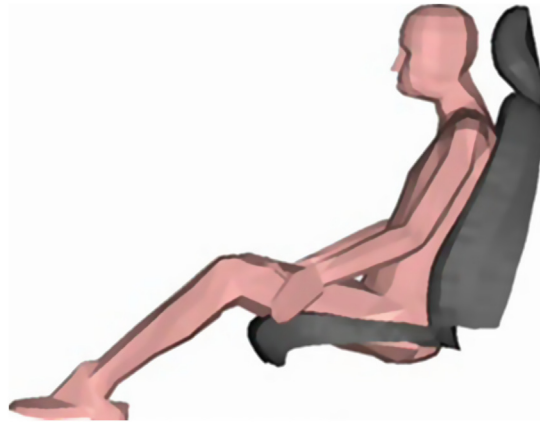
FIGURE 19.15 Full-body biomechanical human model interacting with a car seat, where seat and soft-tissue compliance is modeled using stress-penetration curves.
