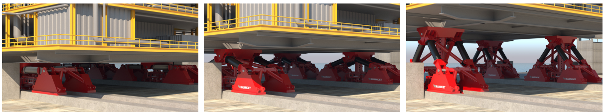
Figure 7.7: Internal jacking with the RDSF system
