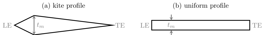
Figure 2: Schematic diagram of two cross-sectional profiles that are used to describe the chordwise mass distribution. The maximal thickness of the cross-section is denoted as t_m . LE and TE represent the leading edge and trailing edge, respectively.
