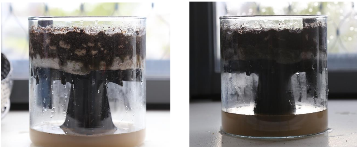
Figure 84: First test attempt results: TGS upper light substrate, TGS lower light substrate (own work)
