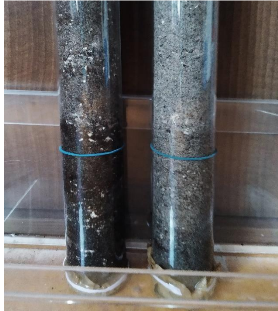
Figure 104: capillary rise, lower light substrate on the left and upper light substrate on the right
