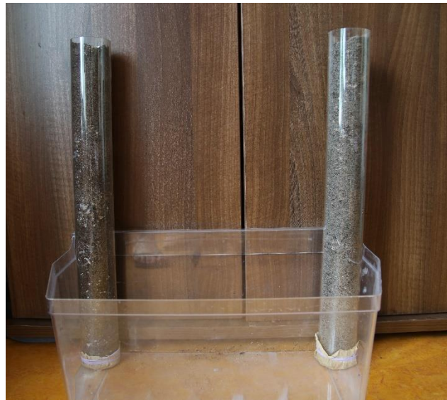
Figure 98: Capillarity experiment/ lower light substrate on the left and upper light on the right (own work)
