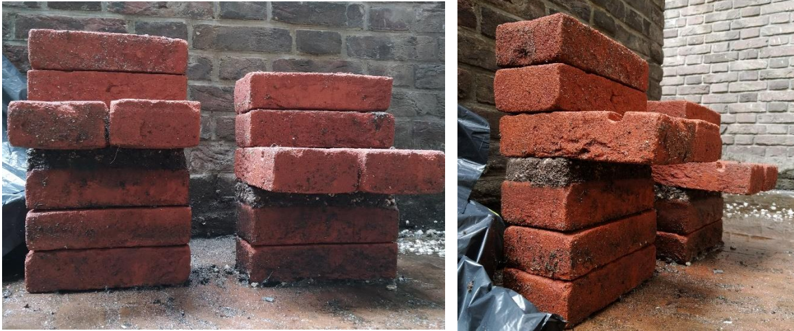
Figure 92: Wall part on the left composed with TGS lower light substrate and wall part on the right with TGS upper light substrate (own work)
