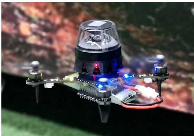
Fig. 1. Tiny, 56-g drone that performs autonomous visual route following with its panoramic camera. We propose an insect-inspired approach to visual route following that allows tiny, resource-restricted robots to follow long routes using only a microcontroller and exceptionally little memory.
