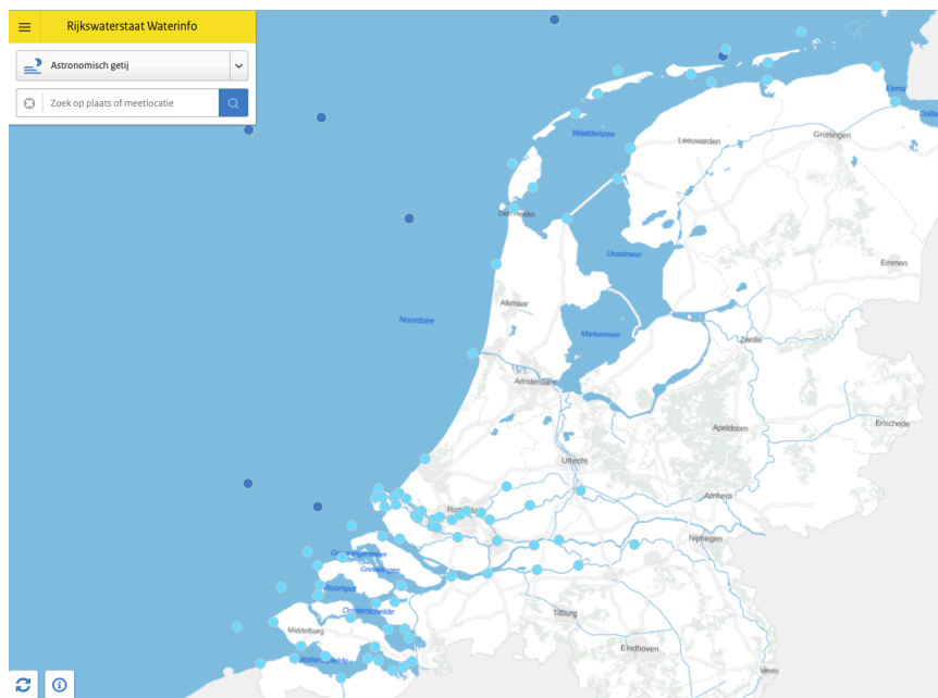
Figure 5.3: Location of gauges at the Dutch coast and inland waterways to check the influence of tidal impact. The influence on the Prinses Beatrix navigation lock is negligible (source: Rijkswaterstaat Waterinfo)
