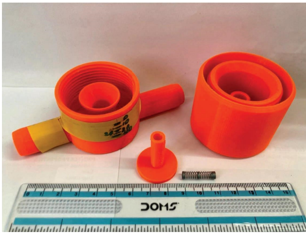
FIGURE 7: 1st generation design version of the RMT device showing valve plunger, valve body, spring, and valve cap for adjustment.
