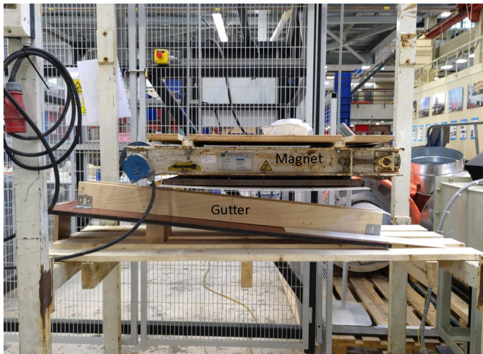
Figure 2.13: The modified overbelt magnet used during the experiments.
