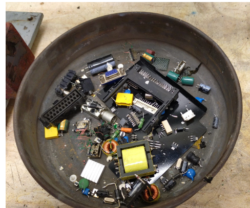
Figure 2.3: An example of a filled collection pan from the component removal step.
