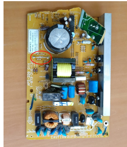
Figure 2.2: An example of a damaged CRT PCB, direct connection is marked by the red circle.
