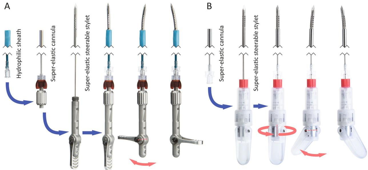
**Figure 1.** Modular designs of v1 planar (A) and v2 omnidirectional (B) steerable needles, with hydrophilic sheaths and nitinol stylets and cannulas. Compliant joints enable tip articulations of approximately  $11^\circ$ . Assembly steps are shown with blue arrows, and degrees of freedom in actuation with red arrows.
