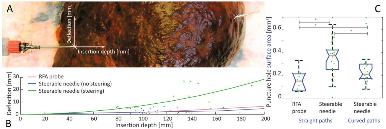
**Figure 3.** Illustration of insertion depth and needle deflection (A), and summary of deflection data (B) for punctures in fresh, cirrhotic liver explants, using the RFA probe and steerable needle v2, along straight and curved paths. Also shown are summary boxplots and individual data points (C) of histological tissue damage ( $\text{mm}^2$ ) after the insertions. The asterisks indicate Wilcoxon rank sum test differences ( $\alpha=0.05$ ).
