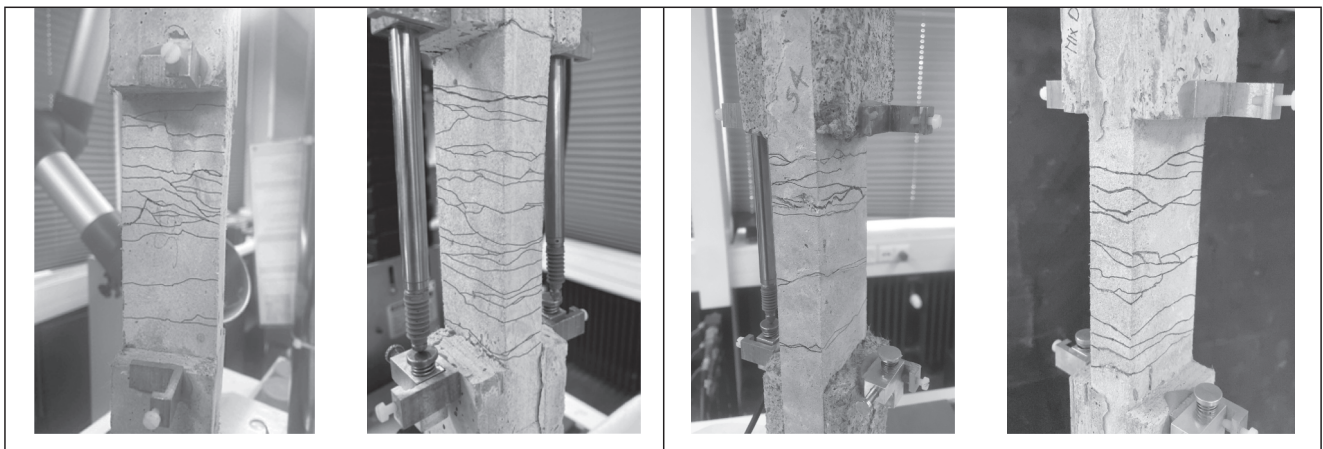
Fig. 22. Representative samples for the cracking patterns of the tested mixes.
