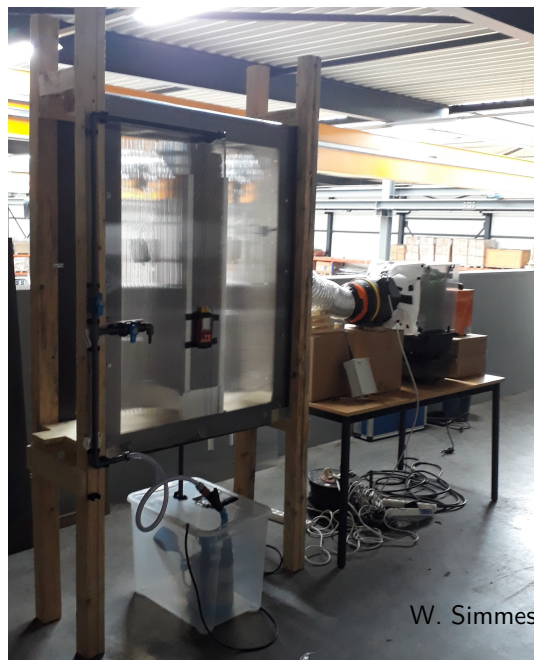
(d) Complete setup with fan, evaporator and heater.
