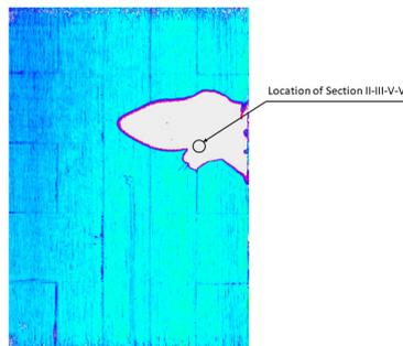
**Figure 5.5:** The failure location of the blended laminate Gomma tested [7].
