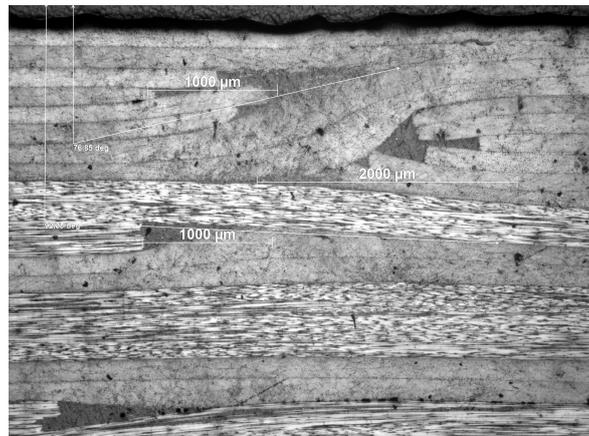
**Figure 4.11:** Through the thickness microscope picture from the upper part of Section I-II. On the left of the picture is Section II and on the right Section I.
