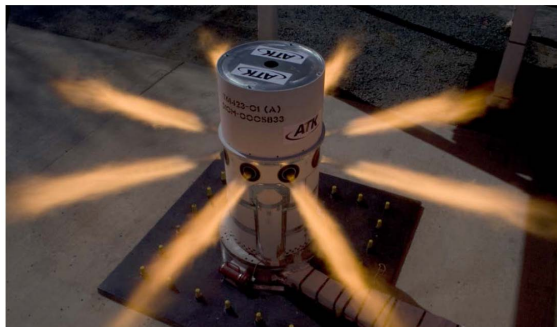
(a) Orion Capsule LAS Attitude Control Motor, from Ref. [3]
