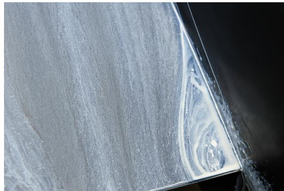
Figure 2.3: Separation near the trailing edge of a wing root, visualised by oil. Image taken from [24].
