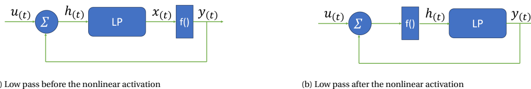
Figure B.1: Two different models of creating a continuous time recurrent neuron.
