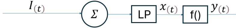
Figure 3.2: Example schematic of a single continuous-time feedforward neuron. I(t) denotes the time-varying input to the neuron, x(t) the low-pass filtered input, i.e. the state of the neuron, and y(t) the output of the neuron after nonlinear activation.
