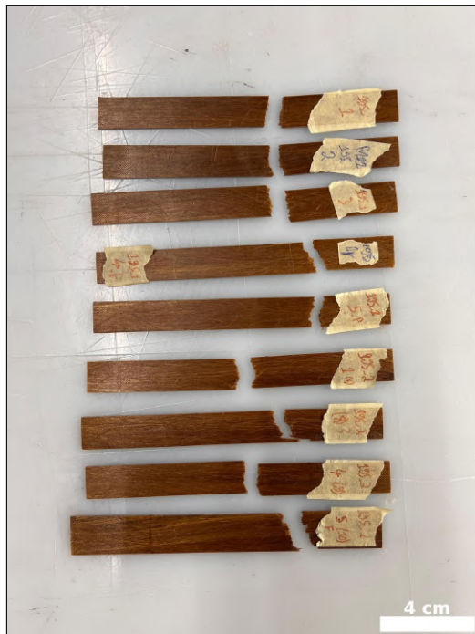
Figure 5.9: Failure of PA11 195 samples
