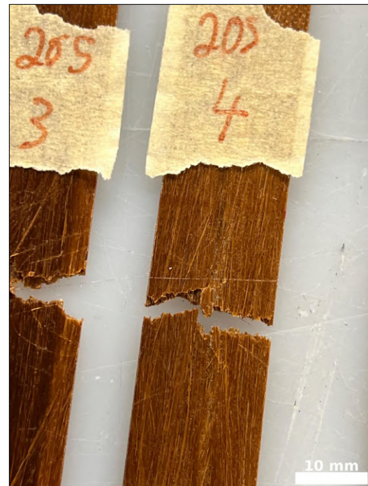
Figure 5.10: Failure of PA11 205 sample
