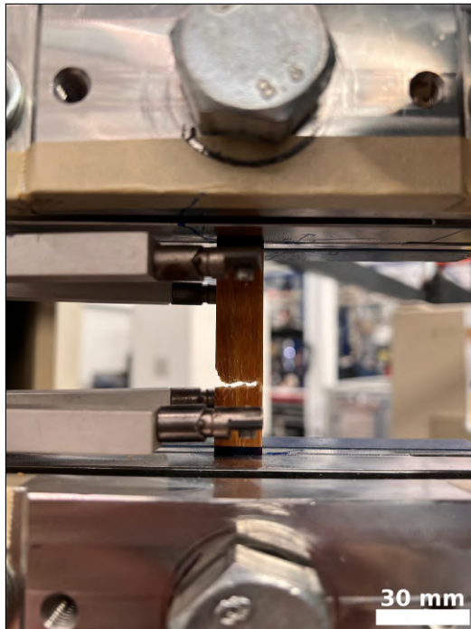
Figure 5.3: Failure of epoxy sample in UTM
