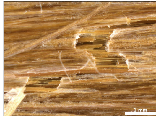
Figure 5.6: Failure of PP 180 sample 1 [5X zoom]
