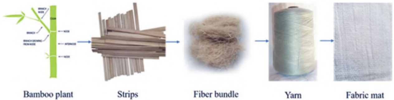
Figure 1.1: Flowchart of the full extraction process from Bamboo plant to fabric [1]
