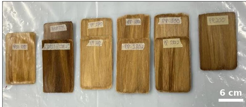
Figure 4.7: Composite plates produced by compression moulding
