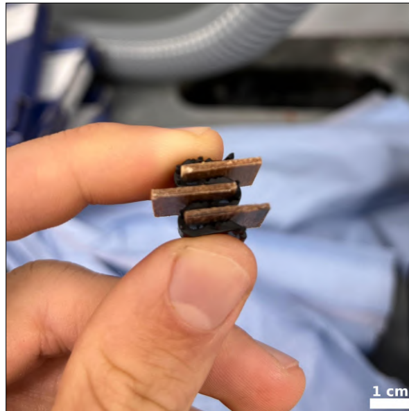
Figure 4.14: Cut samples pieces clamped in holder
