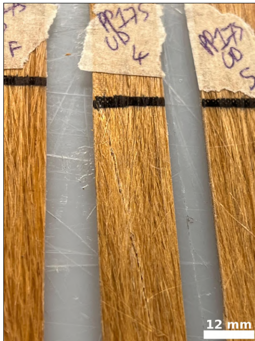
Figure 5.5: Failure of PP UD sample
