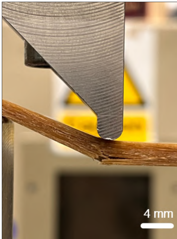
Figure 5.15: Tensile fibre fracture epoxy flexural sample [3X Zoom]
