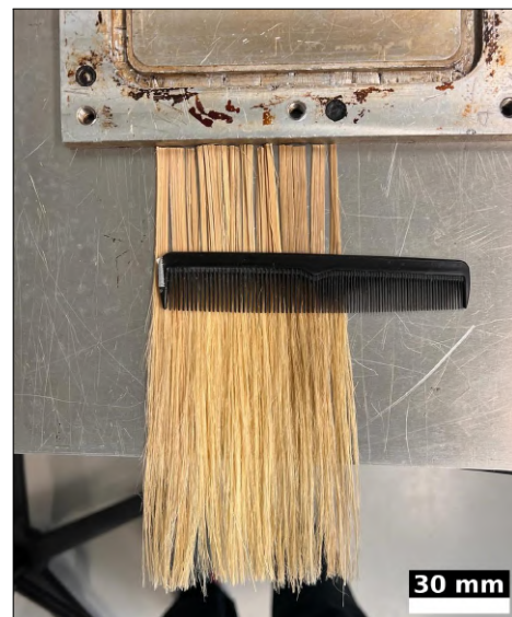
Figure 4.5: Fibre combing process
