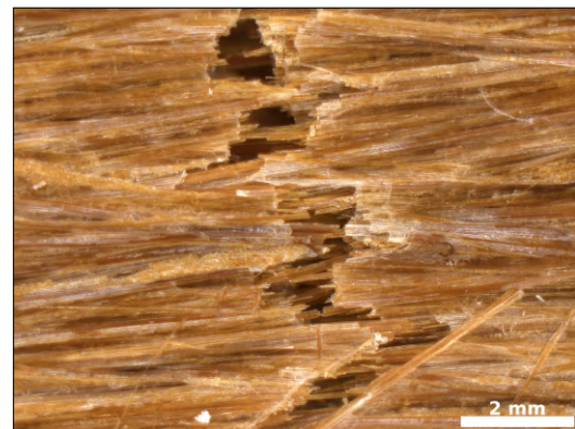
Figure 5.8: Failure of PP 210 sample
