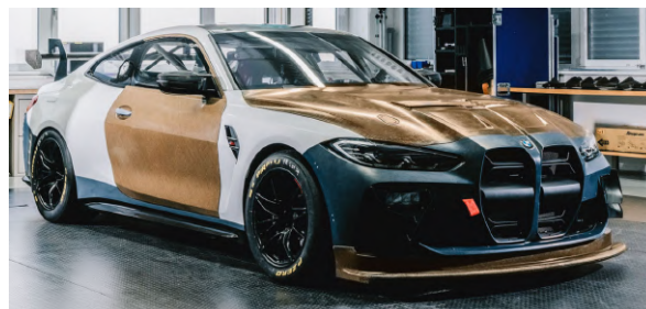
Figure 8.3: Usage of natural (Flax) fibre in motorsport bodywork parts. Source: BCOMP
