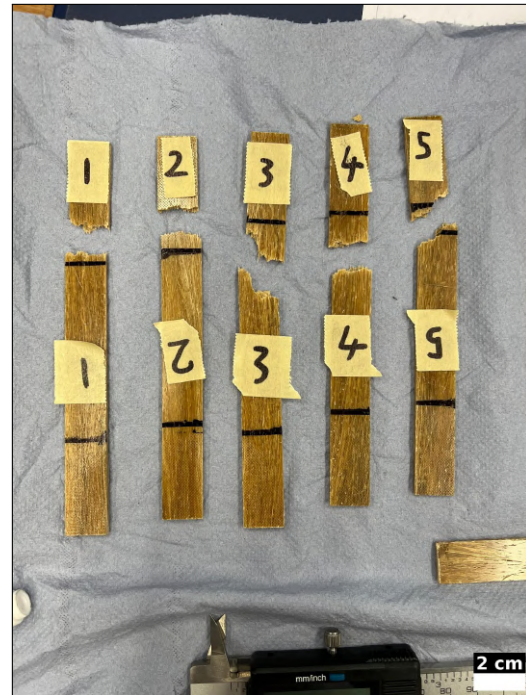
Figure 5.4: Failure of epoxy samples 1 to 5
