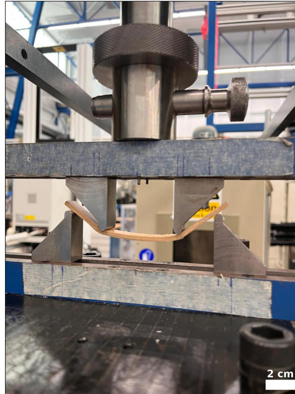
Figure 4.12: Flexural testing: 4PB set-up [Zoom 0.5X]
