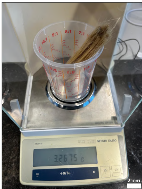
Figure 4.4: Fibre weighing on scale
