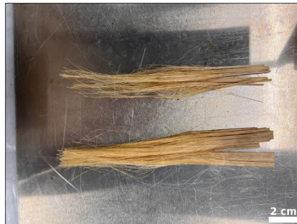
Figure 4.3: Fibre selection: insufficient fibre bundle (top) and selected fibre bottom (bottom)
