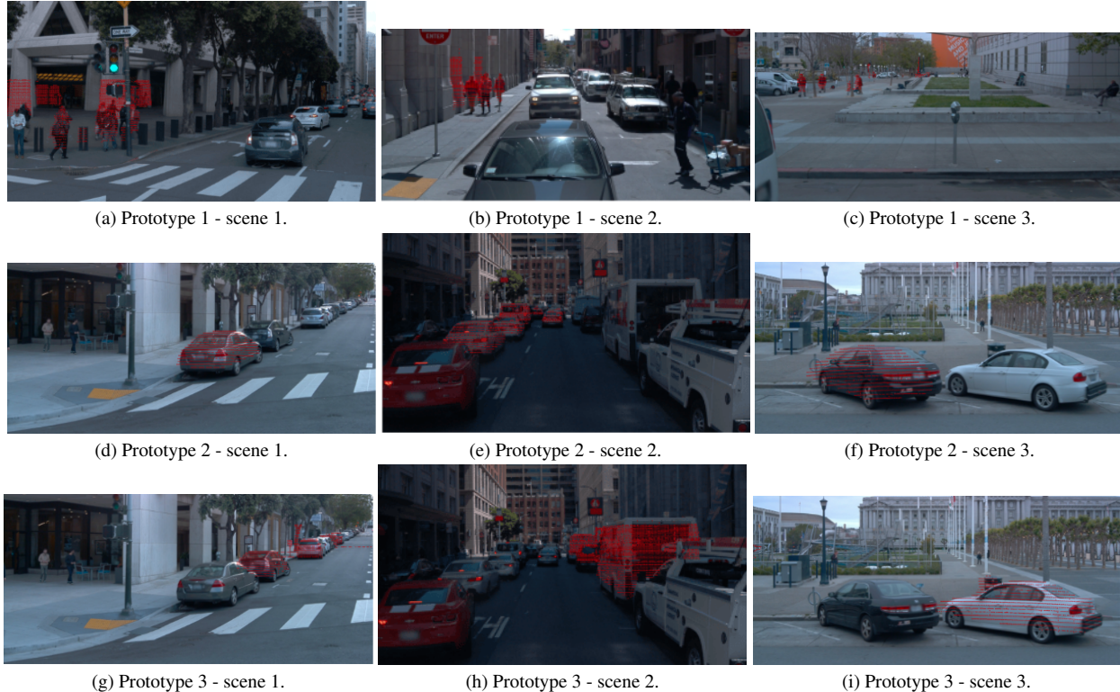
Figure 13. Qualitative visualisation of the semantic features captured by the prototype embeddings. The projected cluster points (as shown in red) within the images correspond to a spatial cluster that was semantically similar to one of the prototype embeddings. The rows in the figure correspond to the 3 prototype embeddings while the columns correspond to 3 different scenes chosen from WOD.
