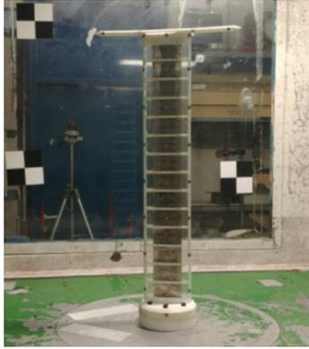
**Fig. 1.** Pazy wing installed vertically in the wind tunnel test section at the Technion [1]
