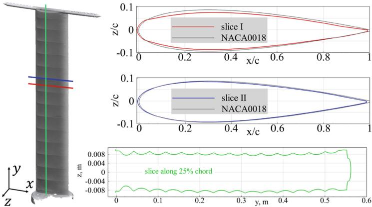
**Fig. 2.** Shape scan of the outer geometry of the Delft-Pazy wing
