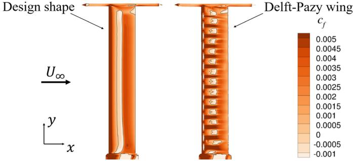
**Fig. 3.** Comparison of skin friction coefficient distributions at  $\alpha = 4^\circ$  angle of attack
