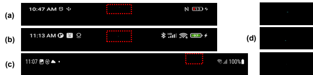
Figure 10: Screenshots of the smartphone status bar when running the one-pixel perturbation on (a) ZTE AXON30, (b) Xiaomi MIX4, and (c) Samsung Fold4. The TSR is highlighted by the red dotted rectangle, and magnified in (d). These changes are imperceptible.
