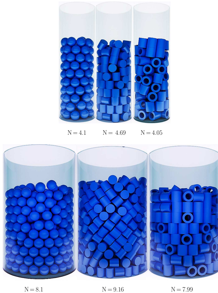
Fig. 3.15 Examples of RBD-simulated structures of spheres, cylinders and Raschig rings.
