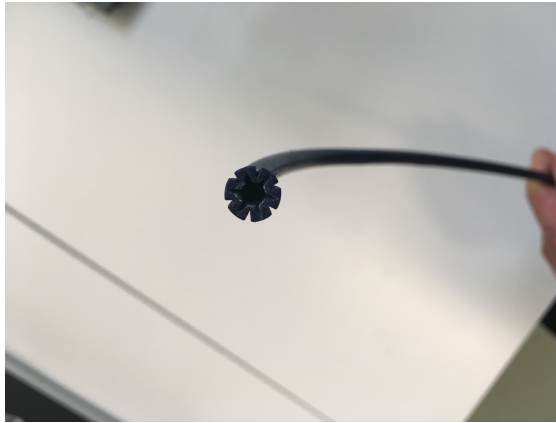
Figure 2.5: The tip of the Edwards delivery system in which the stent is placed to provide support
