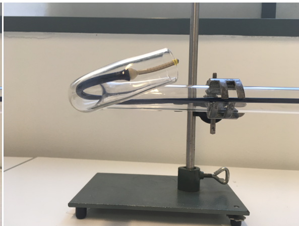
Figure 3.17: Showing the orientation of the prototype in the aorta model in the sagittal plane.
