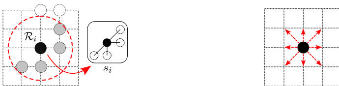
(a) Example of a local state s_i \in \mathcal{S} of a robot \mathcal{R}_i . The robot is shown in black and its neighbors within sensing range are shown in gray. It is assumed that a robot can always sense neighbors in the 8 grid points that surround it.
