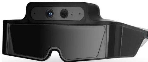
Figure 6. Optical see-through HMD – META Spaceglasses ( https://www.spaceglasses.com/ ).
