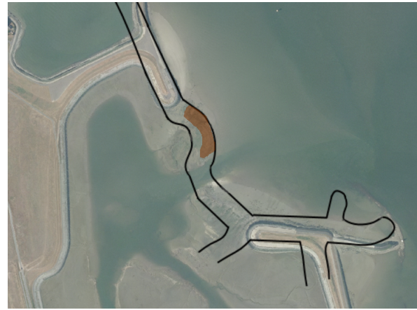
(b) Top view of inlet from aerial photograph in 2019. Old dyke layout from 1850 is shown in black contour lines and the location of remains of the old dyke is shown in orange. Retrieved from: Atlas van Zeeland.
