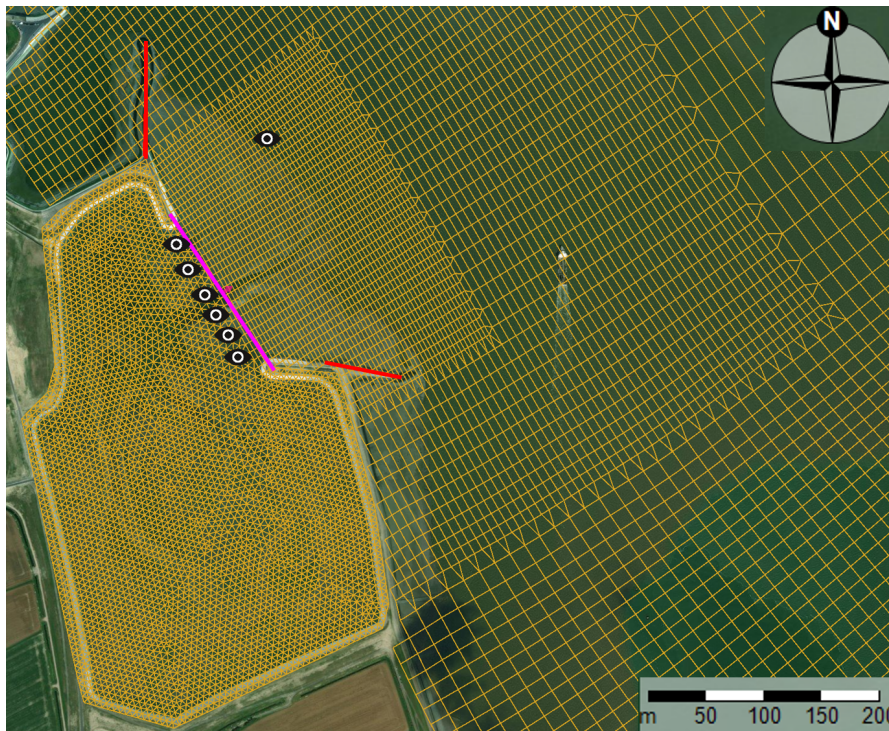
Figure 3.4: Refinement of the grid at the area of Perkpolder. Two mesh refinements are included to move from the regular grid to the triangular grid in Perkpolder. The red lines show the thin dams that represent the groynes. The pink line is an observation cross section to determine discharges. The eye icons represent observation points: the six locations close to the entrance are the locations of the six ADCP sensors and the observation point outside of Perkpolder corresponds with station Walsoorden.
