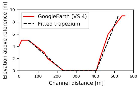
**Figure 4.** Example of approximating a trapezoidal cross section (black) into the Google Earth based cross-section data (red) for virtual station “VS 4” (see also Fig. 1a and Fig. 3). The reference level is equal to the lowest water level in the river profile.
