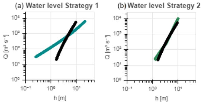
**Figure 11.** Discharge–water-level graphs for the recorded (black) and modelled discharge and stream levels with the optimal model performance ( $E_{NS}$ ) using the Strickler–Manning equation for the discharge–stream-level conversion with cross-section information (a) extracted from Google Earth (Water level Strategy 1) or (b) obtained from a detailed field survey with an ADCP (Water level Strategy 2).
