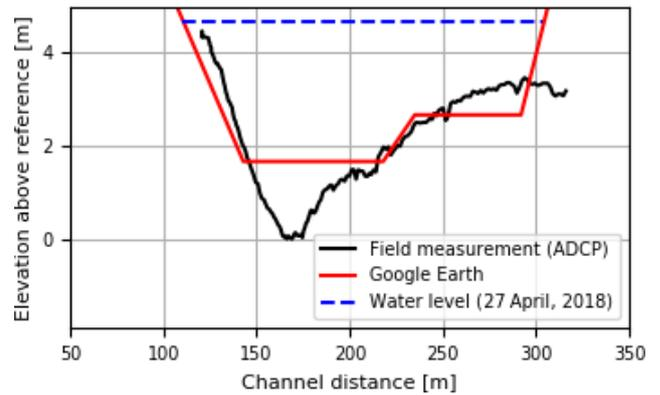
**Figure 5.** River cross section at Luangwa Bridge obtained from Google Earth and detailed field survey including the river water level on 2 June 2008. Field measurements were done with an Acoustic Doppler Current Profiler (ADCP) on 27 April 2018 at the coordinates 30° 13' E and 15° 00' S; the satellite image was taken on 2 June 2008. The reference level is equal to the lowest elevation level measured with the ADCP.
